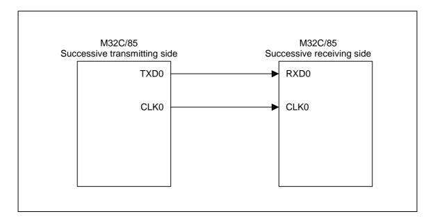
Figure 1. Example Connection for Successive Transmission/Reception
