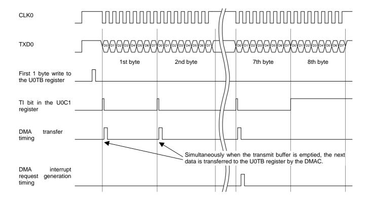
Figure 2. Successive Transmission/reception Timing
