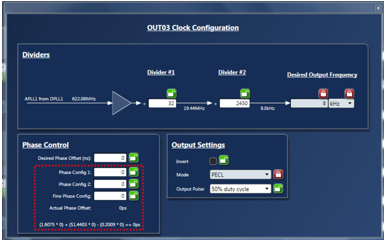
**Figure 6: 82P33831 Timing Commander Output Clock Skew Settings**
