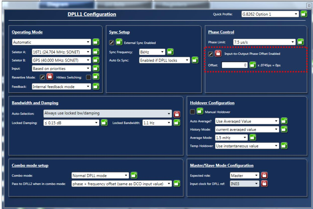
**Figure 4: 82P33831 Timing Commander Input-to-Output Clock Skew Settings**
