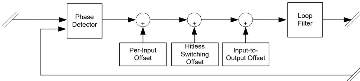
Figure 2: 82P338XX/9XX Input Clock & System Skew Block Diagram
