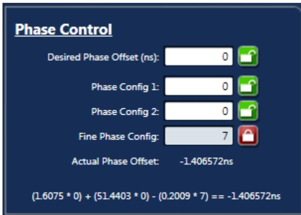
**Figure 8: Output Clock Fine Skew Setting Example**
