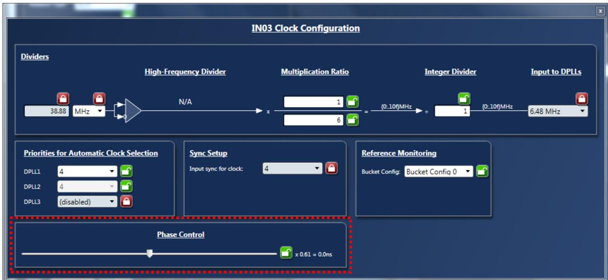
**Figure 3: 82P33831 Timing Commander Input Clock Skew Settings**
