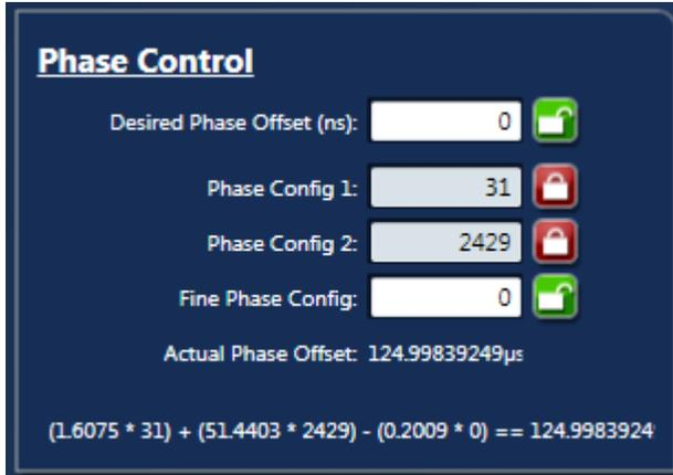
**Figure 7: Output Clock Coarse Skew Setting Example**
