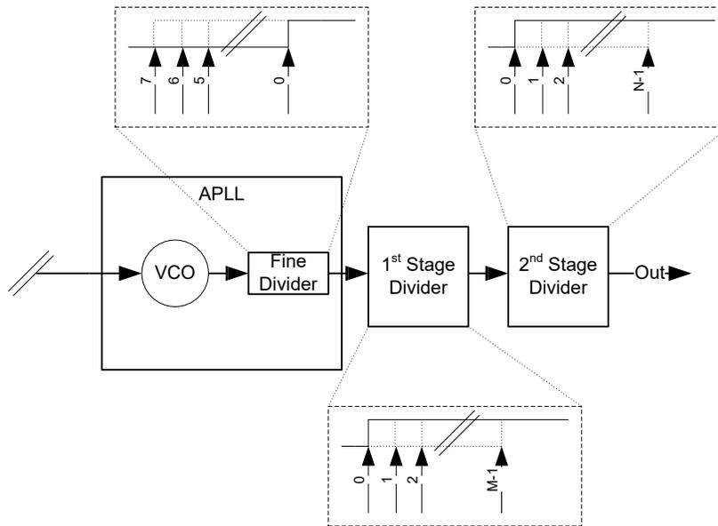
Figure 5: 82P338XX/9XX Output Clock Skew Block Diagram
