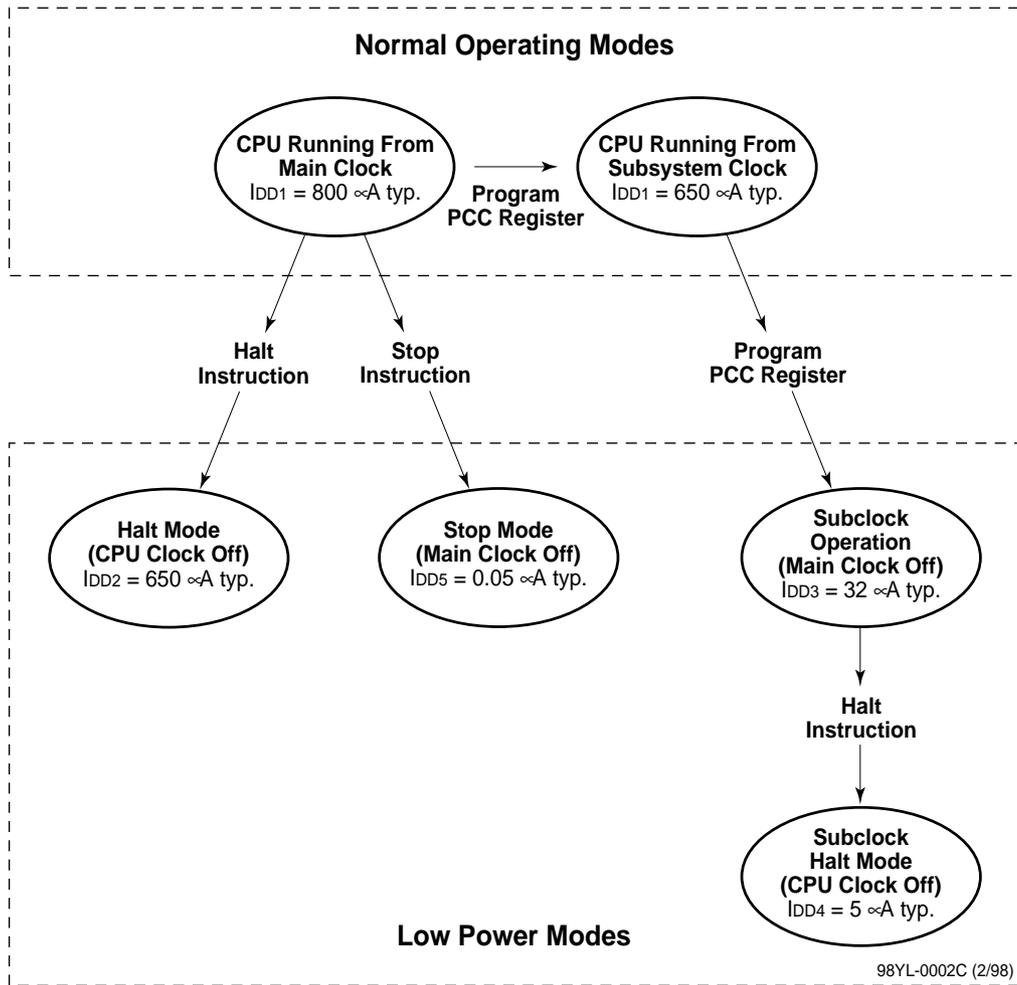
**Note:** Operating current is shown for the  $\mu\text{PD78064}$  at 3 V and 5 MHz.
