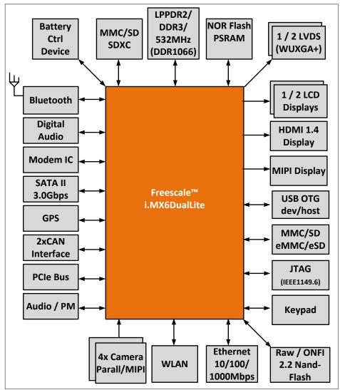
Figure 2: NXP<sup>™</sup> i.MX 6DualLite based system
