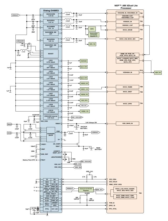
Figure 3: DA9053 / NXP<sup>™</sup> i.MX 6DualLite applications processor example configuration
