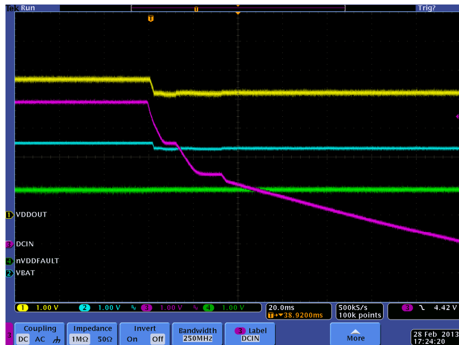
Figure 7 Supply via single diode to provide 4.3V on VBAT
