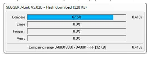
JLink is programming the PE-HMI1 Kit with the Out-Of-Box Demo
