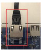
4. Connect the other end of the Ethernet cable to the Power over Ethernet (PoE) supply and plug in the power supply.
