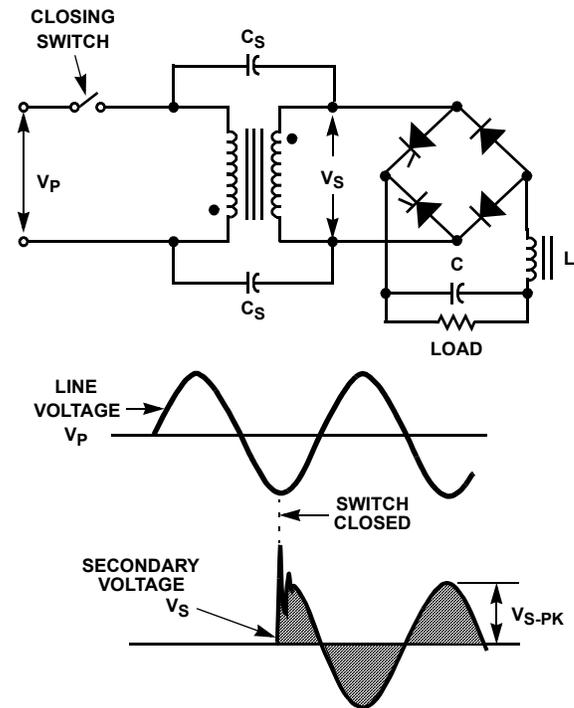
**FIGURE 1. VOLTAGE TRANSIENT CAUSED BY ENERGIZING TRANSFORMER PRIMARY**
