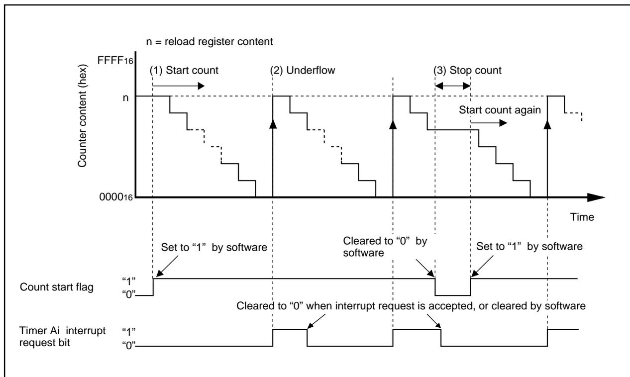
**Figure 1. Operation timing of timer mode**
