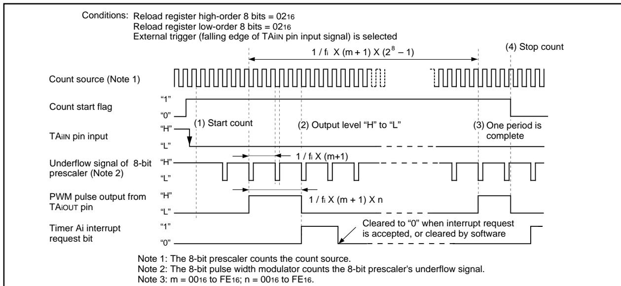
Figure 1. Operation timing of pulse width modulation mode, with 8-bit PWM mode
