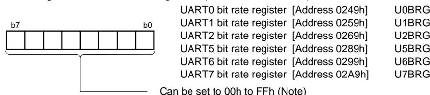
Note : Write to UARTi bit rate register when transmission/reception is halted.
