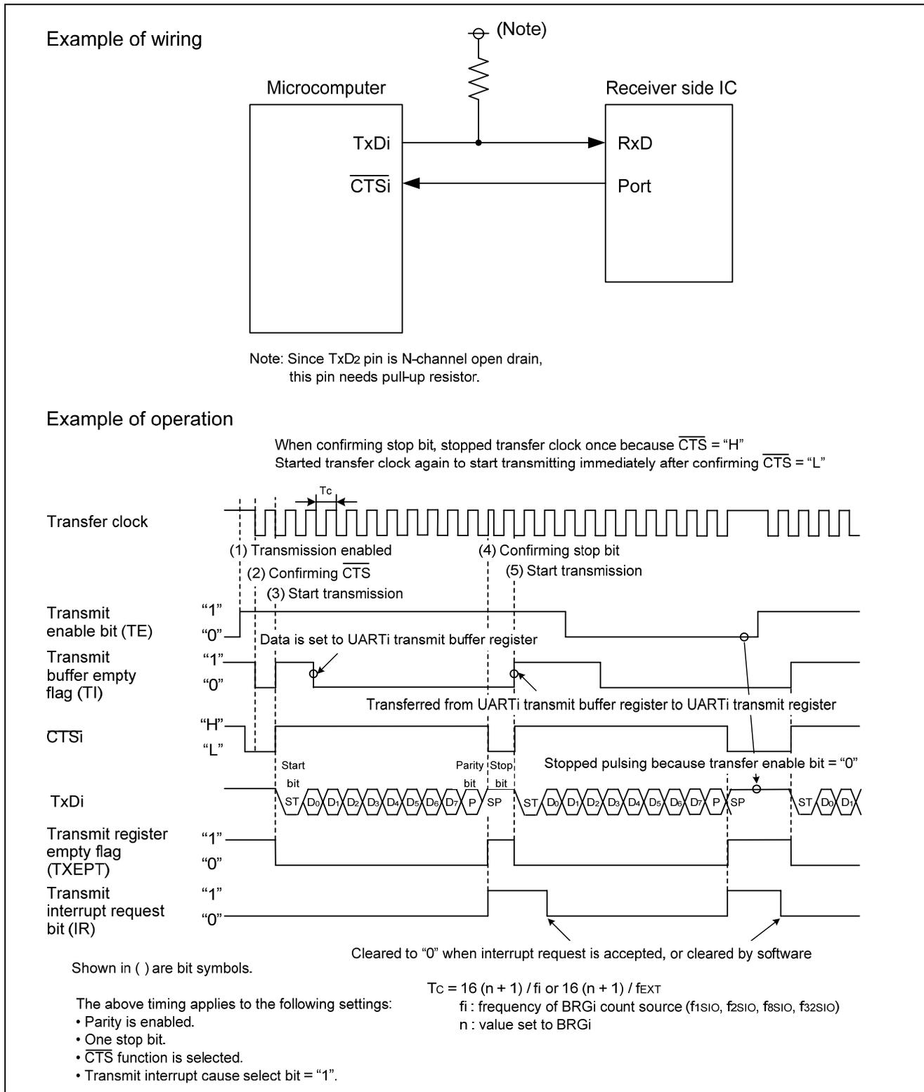
**Figure 1. Operation timing of transmission in UART mode**
