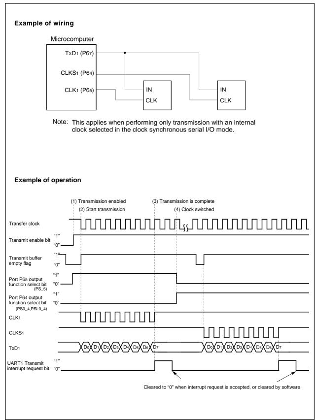
Figure 1. Operation timing of transmission in clock-synchronous serial I/O mode, transfer clock output from multiple pins function selected
