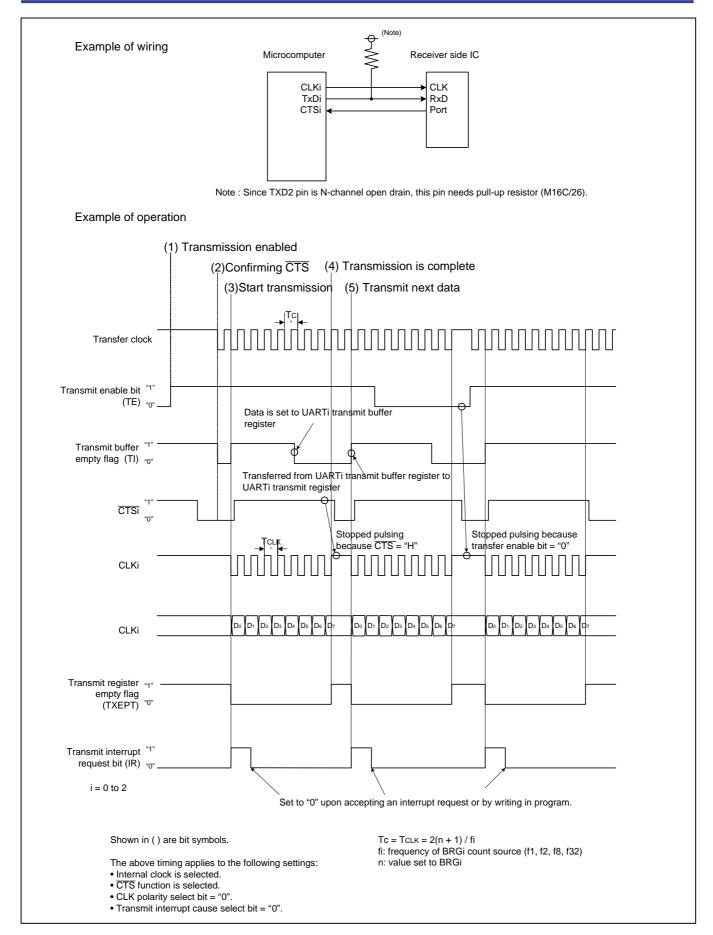
Figure 1. Operation Timing of Transmission in Clock-Synchronous Serial I/O Mode
