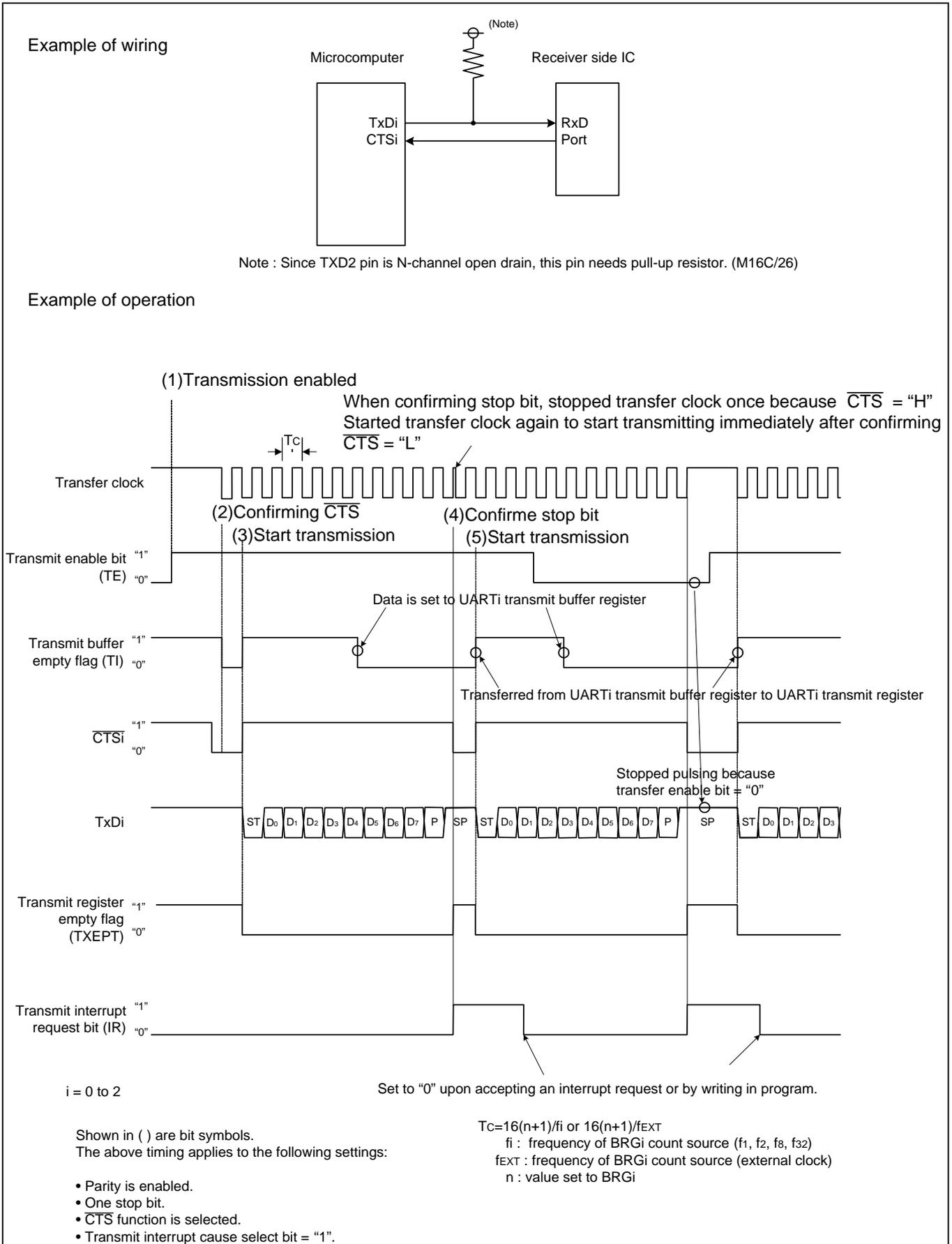
**Figure 1. Operation Timing of Transmission in Clock-asynchronous Serial I/O Mode**
