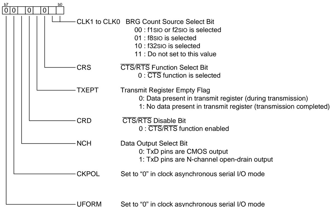
(3) Setting UART2 transmit/receive control register 1
