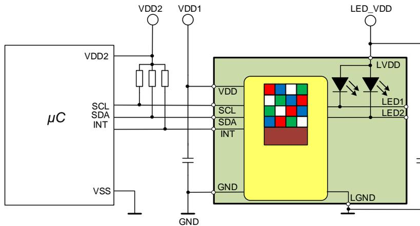
**Figure 1. Application Circuit**
