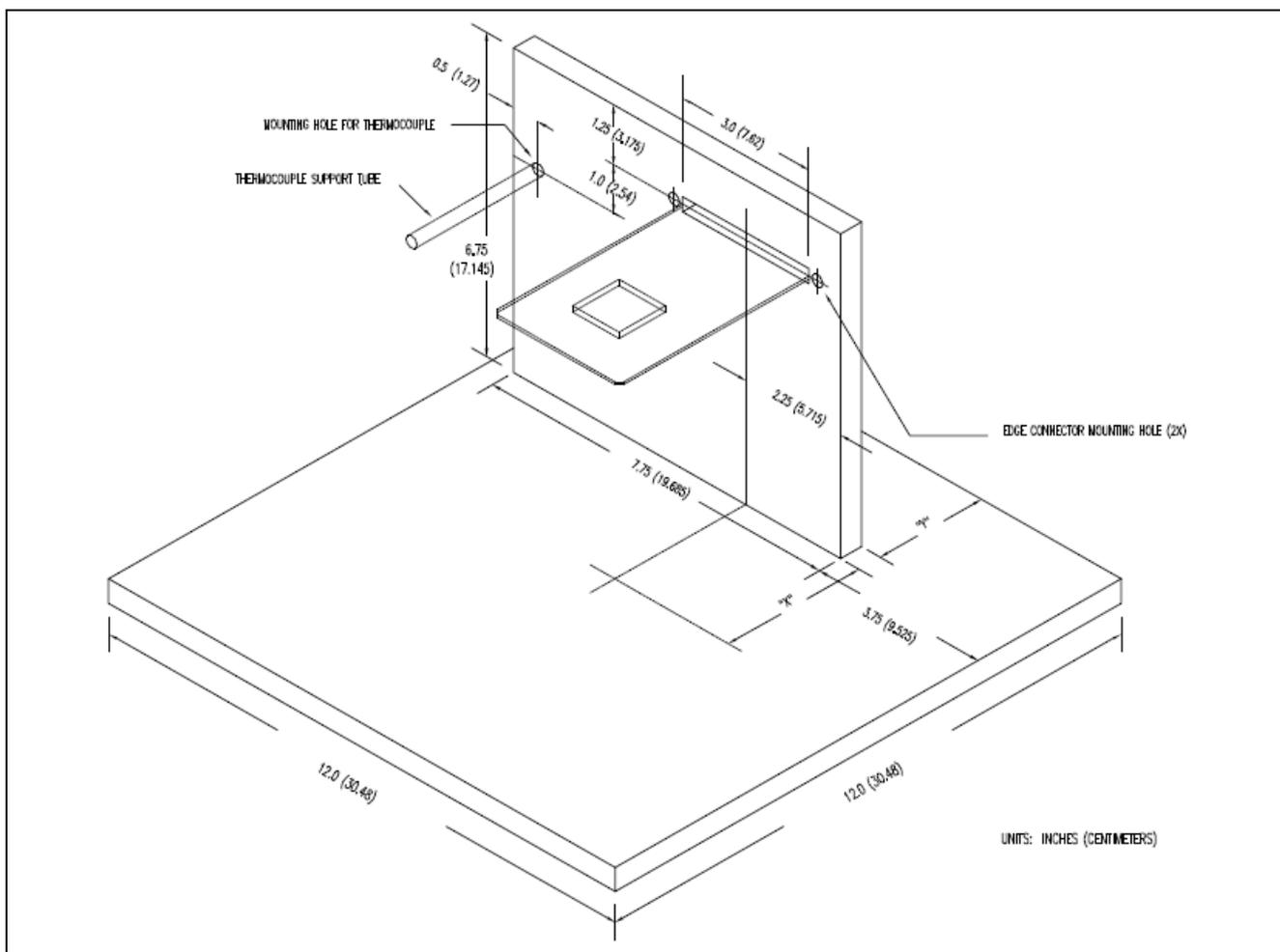
**Figure 2-2 Ta measurement position - bird's eye view (no chassis)
