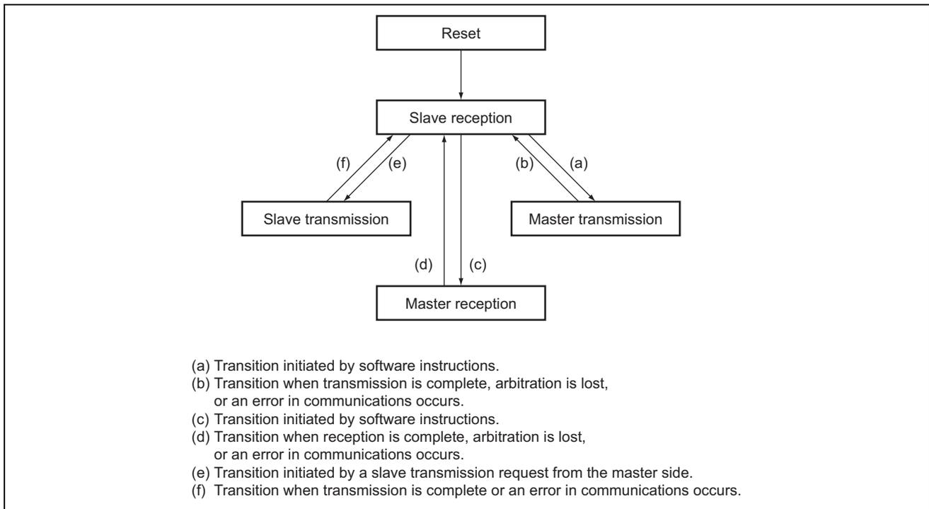
**Figure 7 State Transition Diagram**
