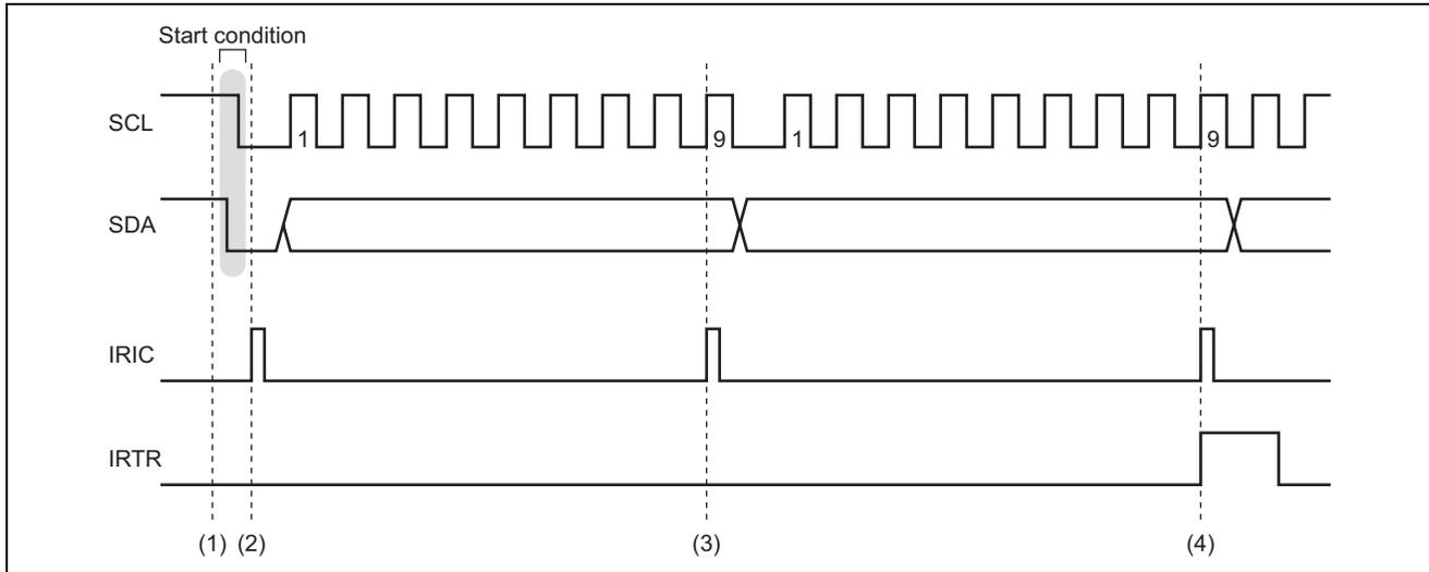
**Figure 3 Timing of Operations in Master Receive Mode**
