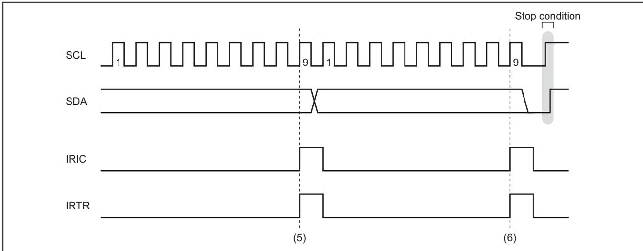
**Figure 4 Timing of Operation of Master Receive Mode 2**
