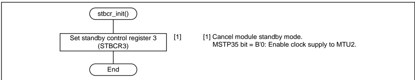
Figure 11 Initialization: Release from Standby
