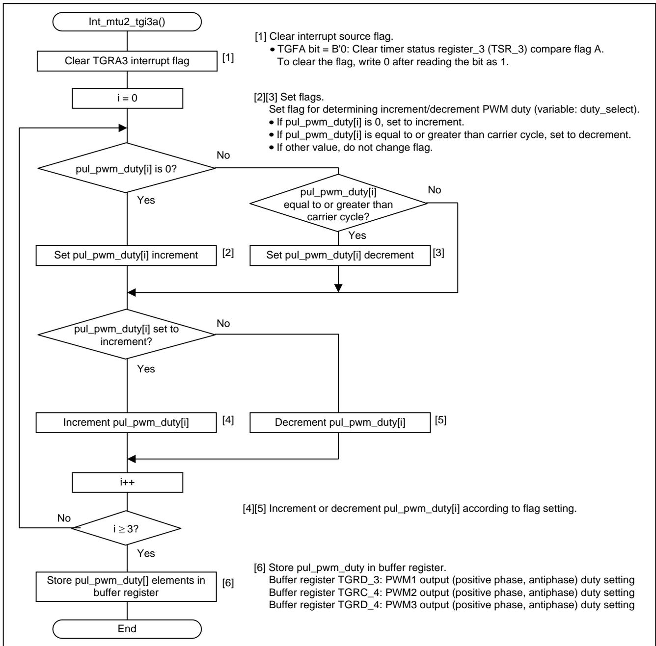
Figure 14 Interrupt Handling
