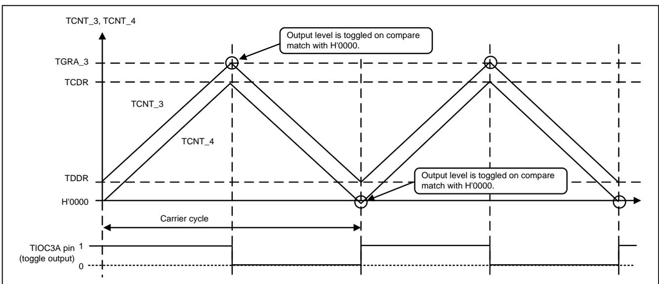
**Figure 8 Operation for Toggling an Output in Synchronization with the PWM Cycle**
