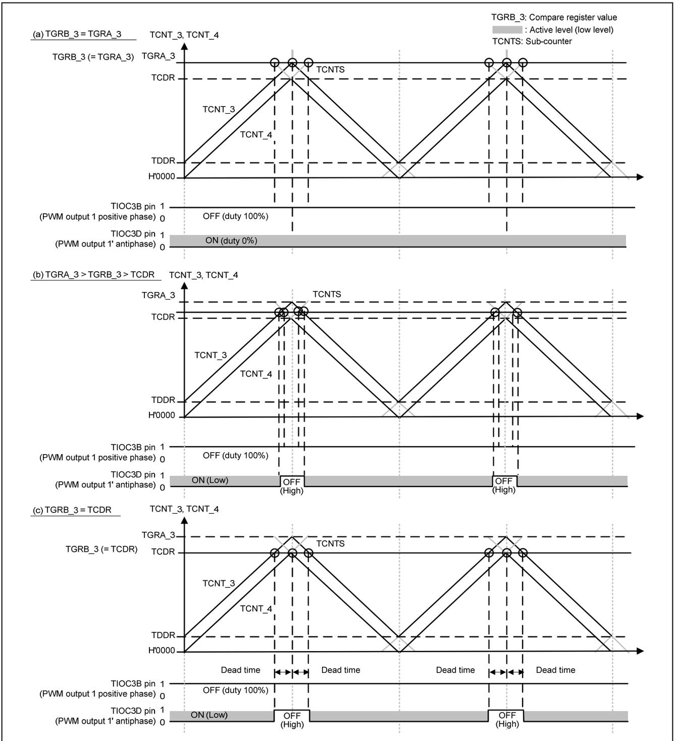
Figure 9 (a), (b), (c) Examples of PWM Waveform Output
