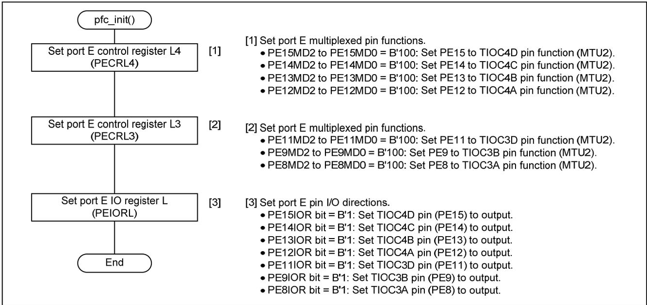
**Figure 13 Initialization of Pin Function Controller (PFC)**
