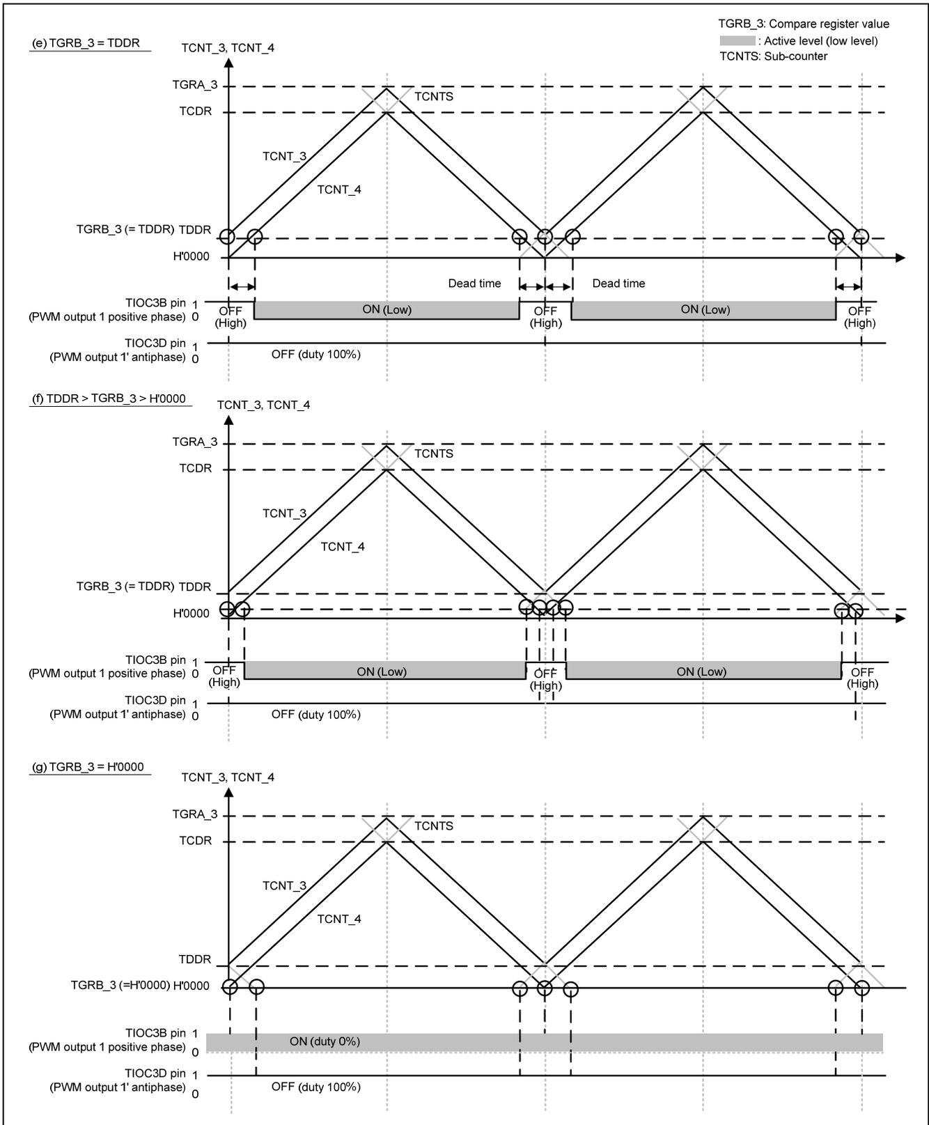
Figure 9 (e), (f), (g) Examples of PWM Waveform Output
