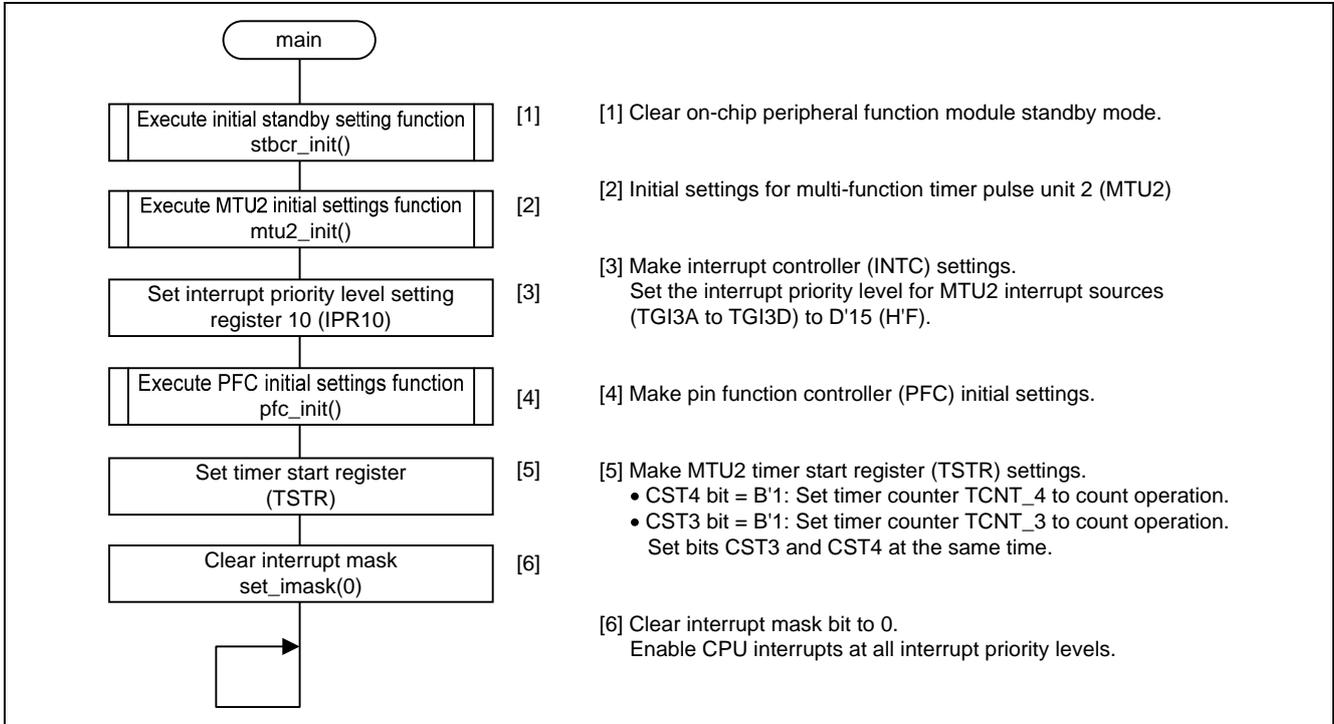
Figure 10 Processing by Function main
