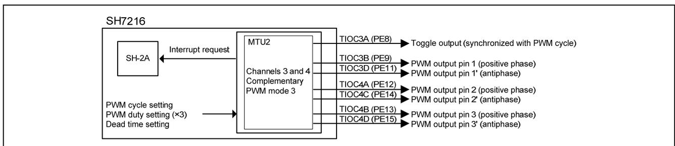
**Figure 1 Three-Phase Complementary PWM Output (Complementary PWM Mode 3)**
