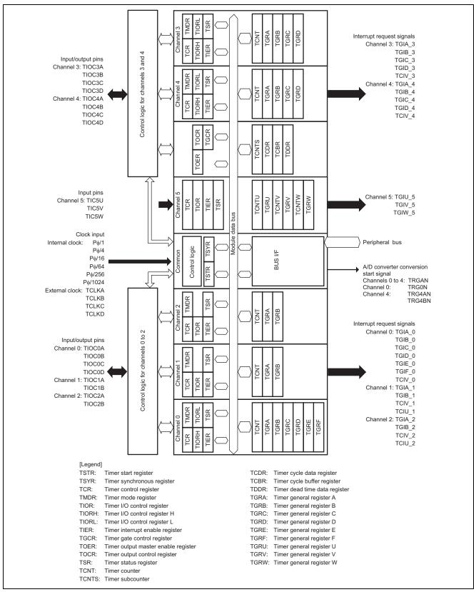
Figure 2 Block Diagram of MTU2
