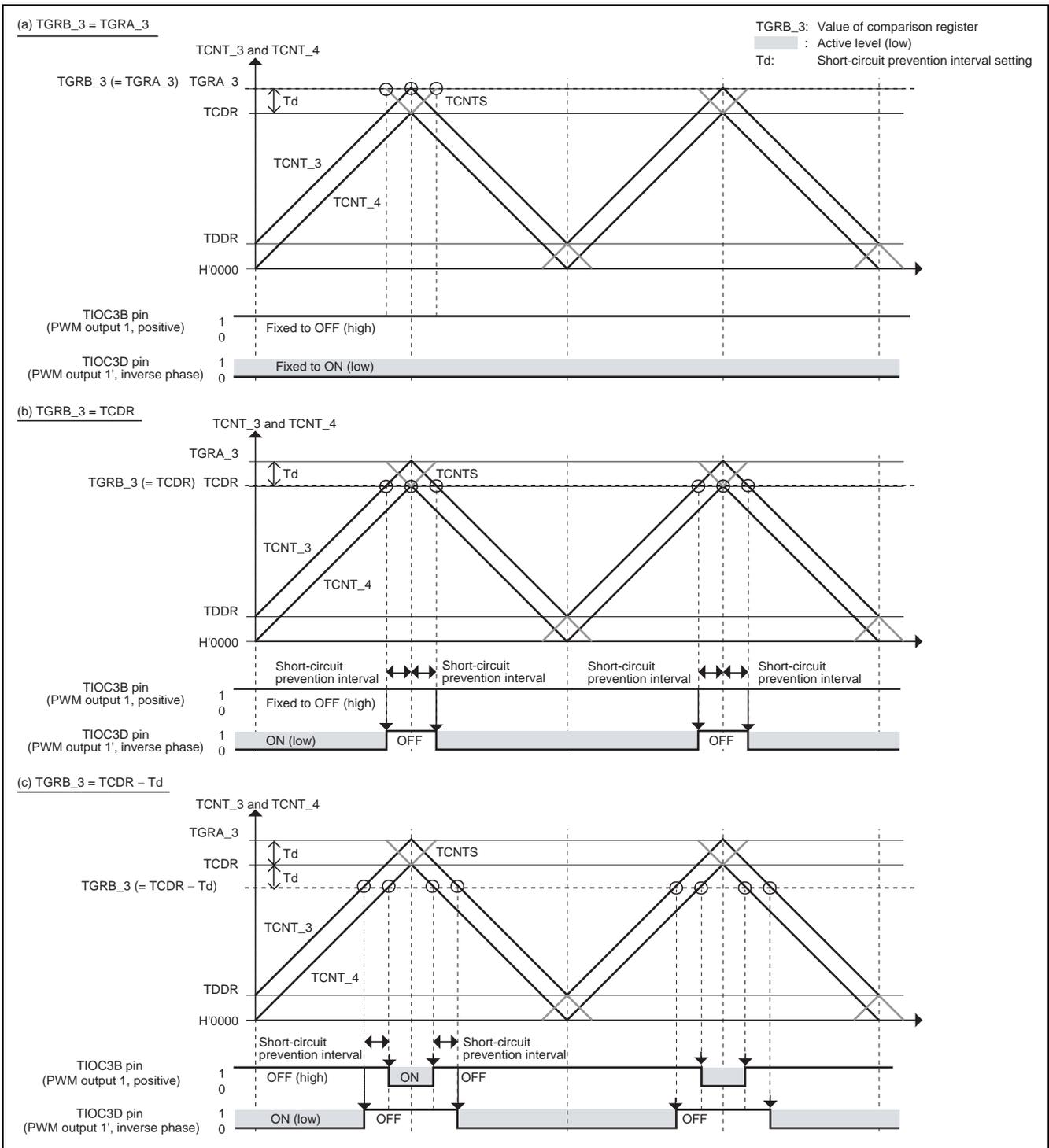
Figure 9 Examples of PWM Waveform Output (1)
