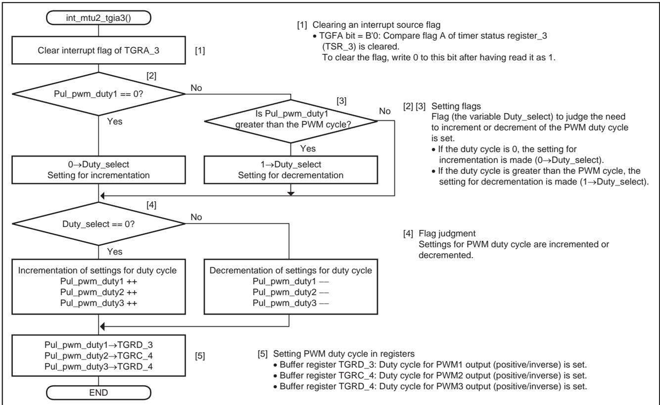
Figure 15 Interrupt Handling
