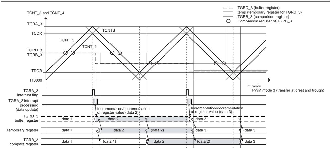
Figure 7 Timing of Updating the PWM Duty Cycle
