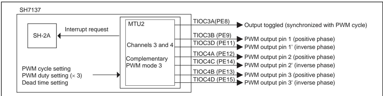
Figure 1 Three-Phase Output of Complementary PWM (Complementary PWM Mode 3)
