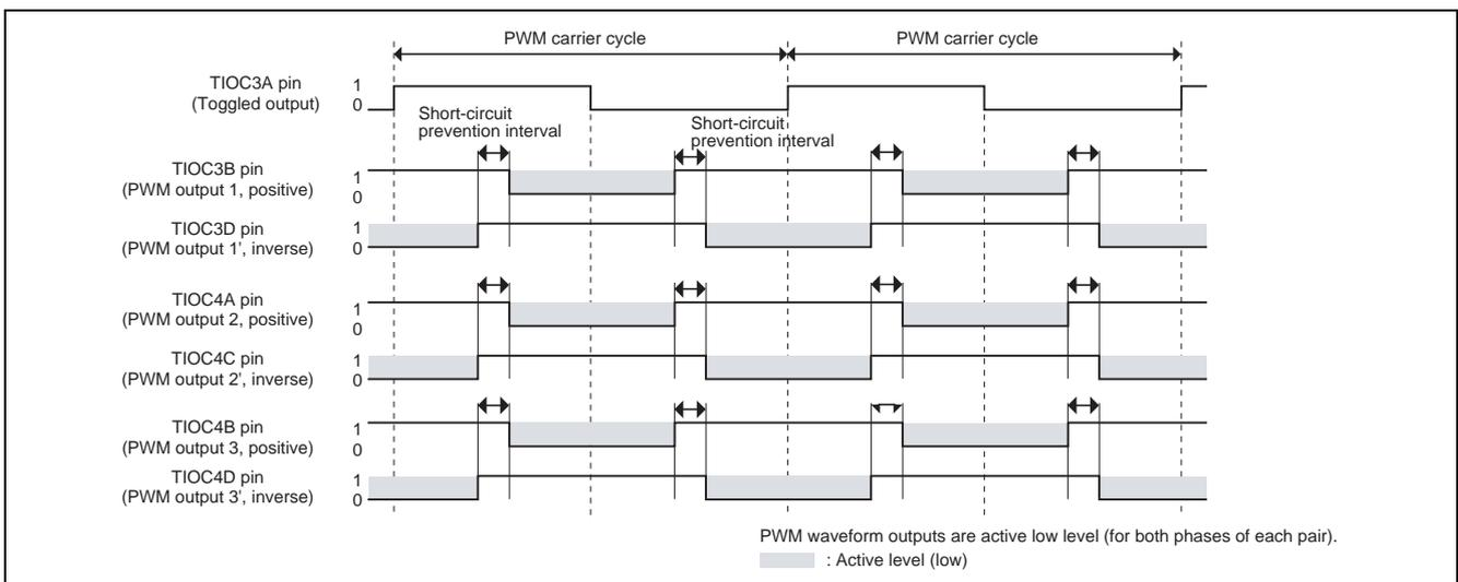
**Figure 4 Output Waveforms in Complementary PWM Mode Operation**
