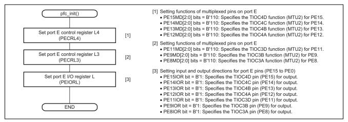
Figure 14 Initialization of Pin Function Controller (PFC)
