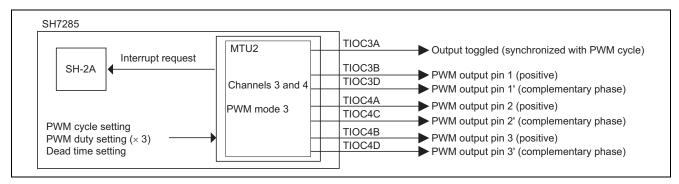
Figure 1 Three-Phase Output of Complementary PWM (Complementary PWM Mode 3)
