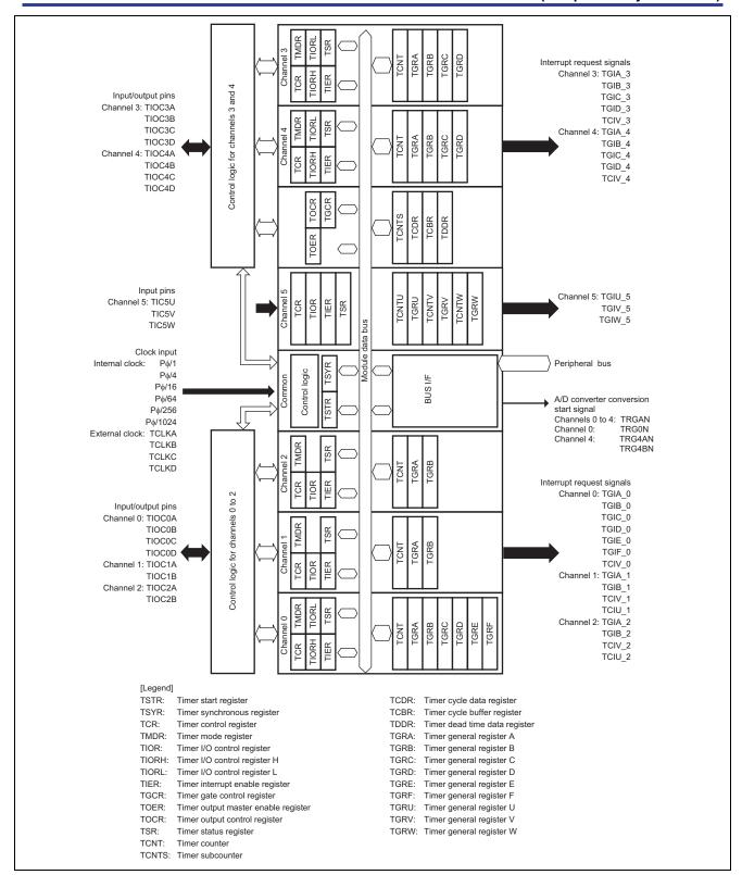
Figure 2 Block Diagram of MTU2
