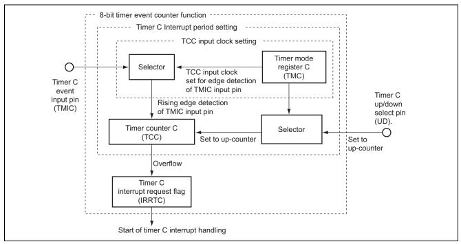
Figure 1 Block Diagram of Timer C Event Counter Function
