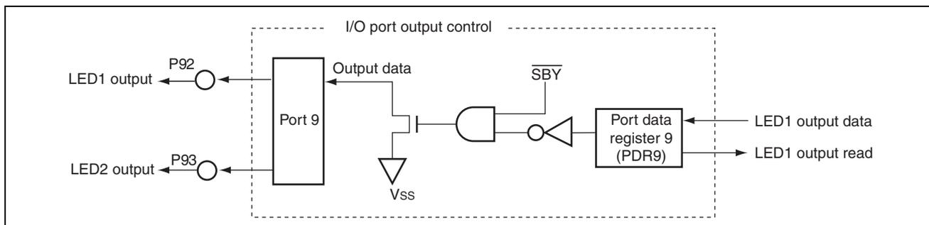
**Figure 2.1 Block Diagram of I/O Port Functions**
