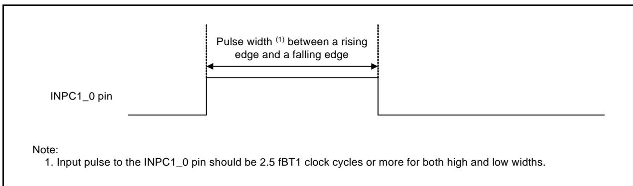
**Figure 5.1** Reference Input Pulse
