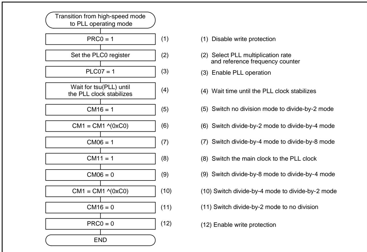
Figure 3.1 Transition from High-Speed Mode to PLL Operating Mode
