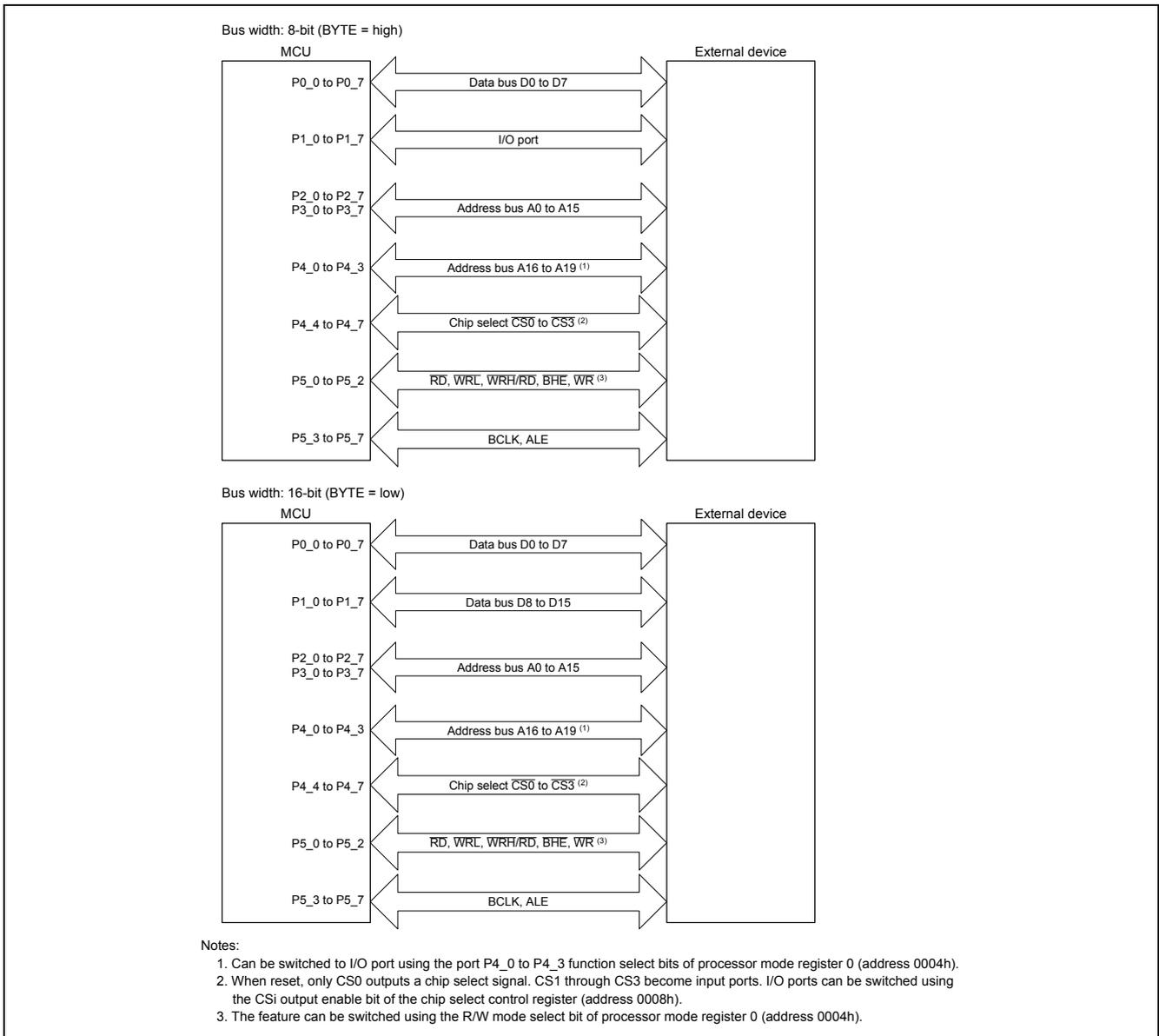
**Figure 3.1 BYTE Pin Level and External Data Bus Width**
