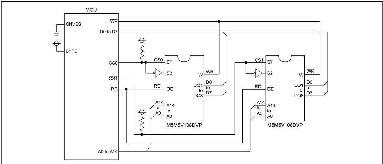
Figure 3.6 Connecting Two M5M5V108DVP's to an 8-bit Wide Data Bus
