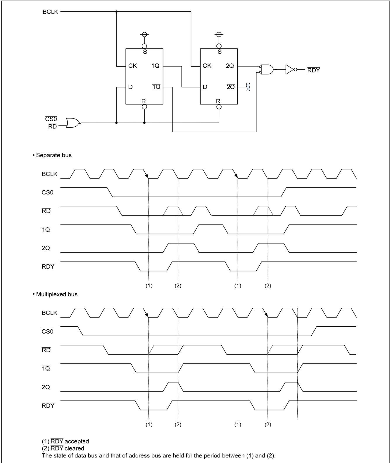
Figure 3.9  $\overline{\text{RDY}}$  Circuit Holding State of Bus for One BCLK  $f(\text{XIN}) = 10\text{ MHz}$
