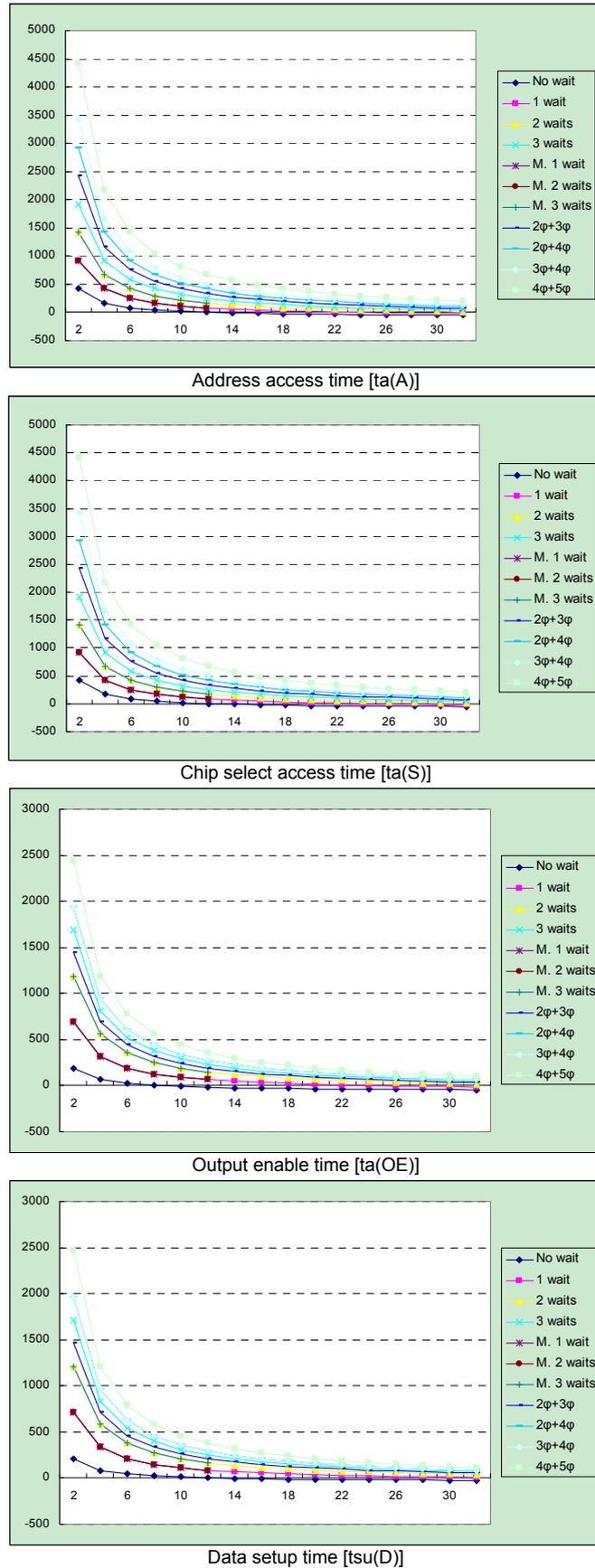
Figure 3.8 Relation between the BCLK Frequency and Memory When Vcc = 3 V
