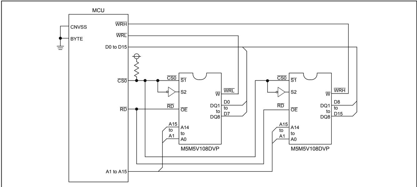
Figure 3.5 Connecting Two M5M5V108DVP's to a 16-bit Wide Data Bus
