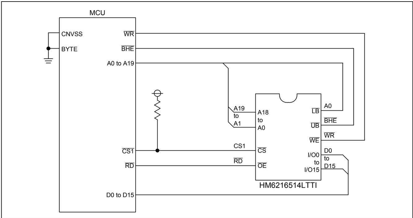
Figure 3.4 Connecting HM6216514LTTI to a 16-bit Wide Data Bus
