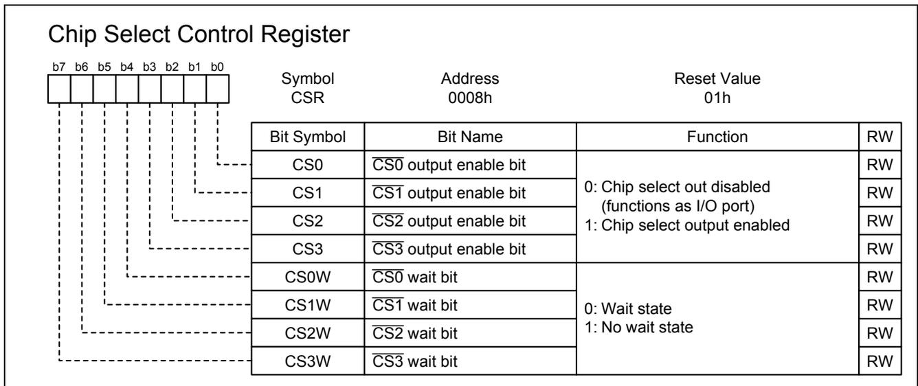
**Figure 3.3 Chip Select Control Register**
