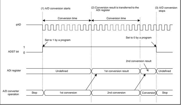
Figure 3.1 Operation Timing in Repeat Mode
