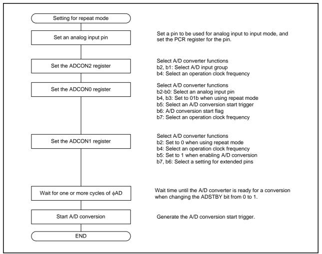
Figure 5.1 Setting Procedure When Using Repeat Mode
