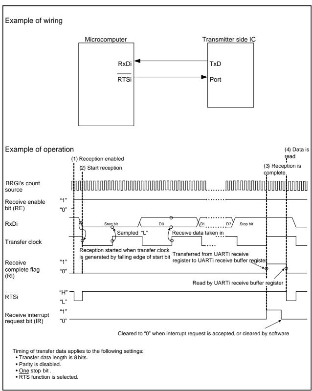
Figure 4.1 Operation Timing of Reception in UART Mode
