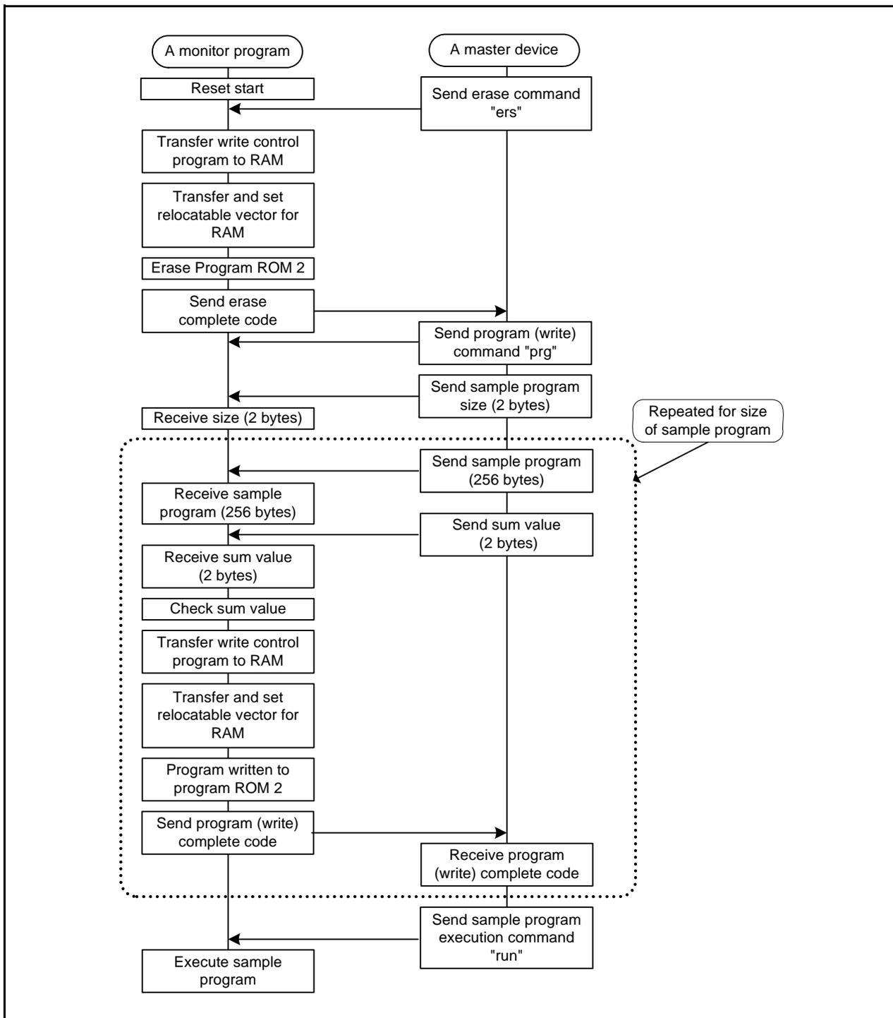
Figure 4.2 Monitor Program Operation Example
