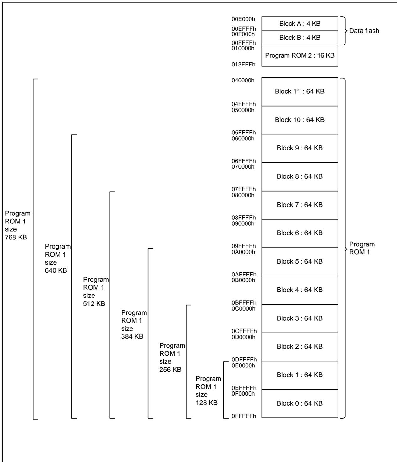
Figure 3.2 Flash Memory Block Diagram
