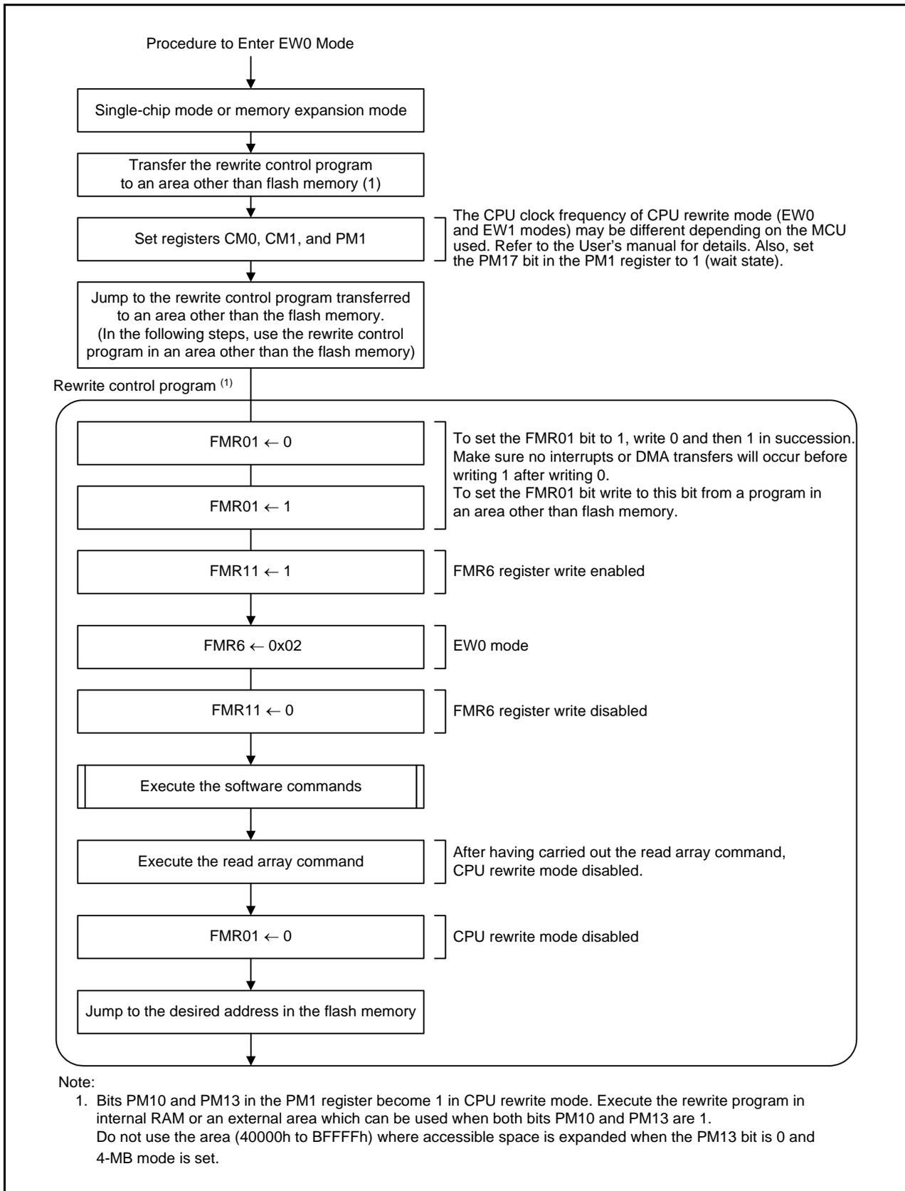
Figure 3.1 Settings and Resetting of EW0 Mode
