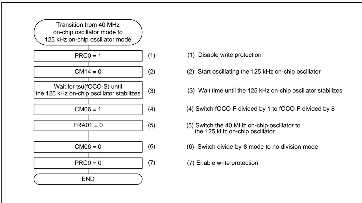
**Figure 3.2 Transition from 40 MHz On-Chip Oscillator Mode (fOCO-F Divided by 1) to 125 kHz On-Chip Oscillator Mode**
