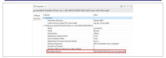
Figure 18. DTC Transfer Start Event Settings in FSP Configurator
