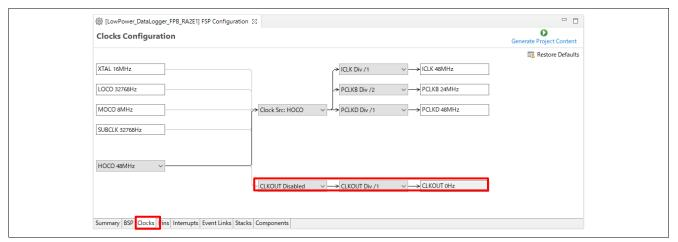
Figure 30. Clock Output Settings in FSP Configurator
