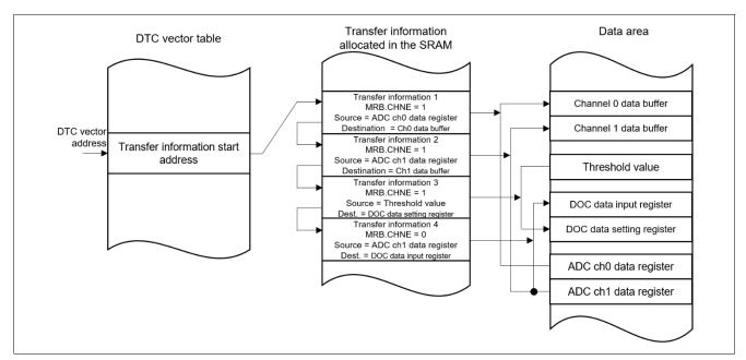
Figure 19. Chain Transfer Operation
