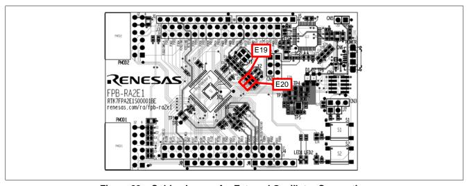
Figure 39. Solder Jumper for External Oscillator Connection
