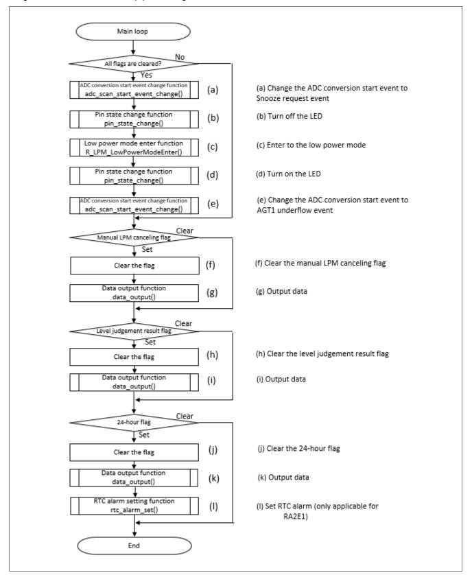
Figure 46. Main Loop Processing
