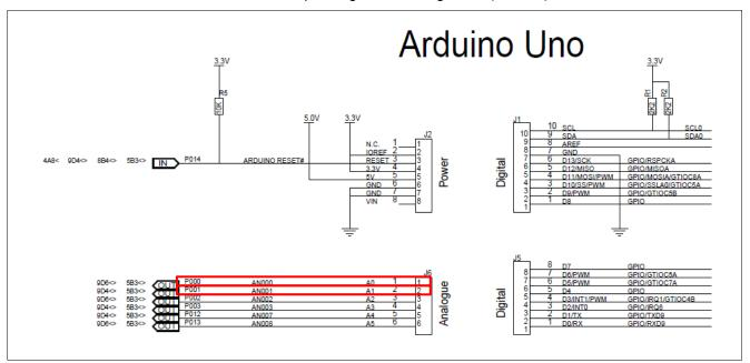
Figure 10. FPB-RA2E1 Kit Arduino-Compatible Connector Analog Signal Pin Connection
