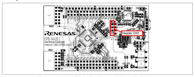
Figure 62. Header CN1 for Force Reset of Onboard E2 Emulator
