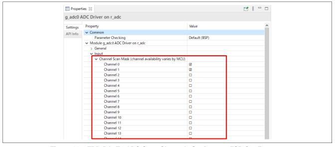
Figure 11. FPB-RA2E1 ADC Scan Channels Settings on FSP Configurator
