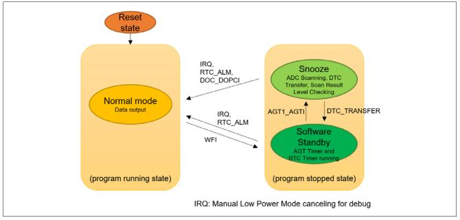
Figure 1. RA2E1 MCU Status and Mode Transition Events
