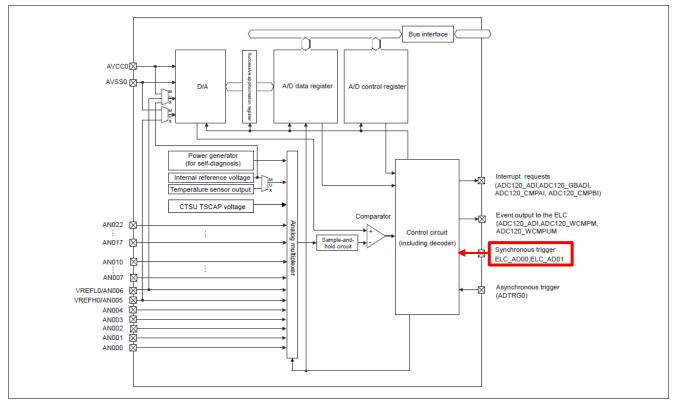
Figure 14. ADC12 Input/Output Events
