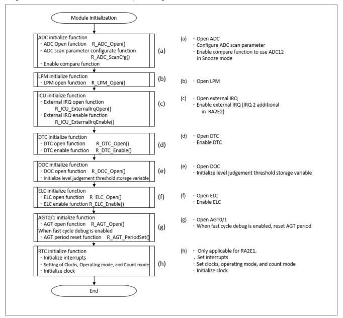
Figure 45. Module Initialization Processing
