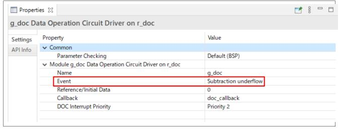
Figure 20. DOC Function Settings on FSP Configurator
