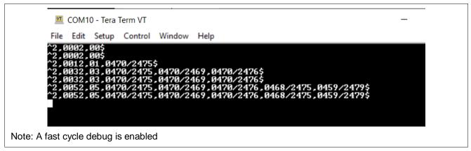
Figure 59. FPB-RA2E2 Example of Data Output Triggered by Pressing the User Switch
