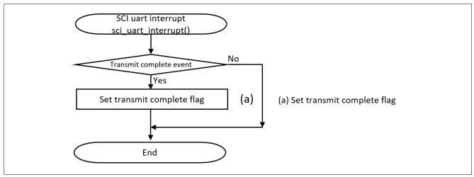
Figure 51. SCI Interrupt Processing
