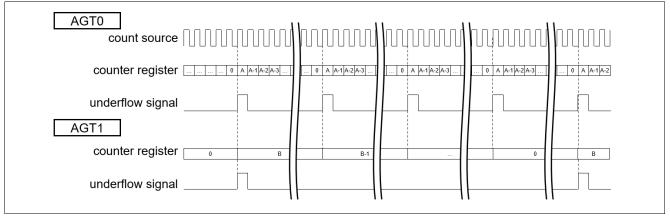
Figure 24. Two-Channel Connected AGT
