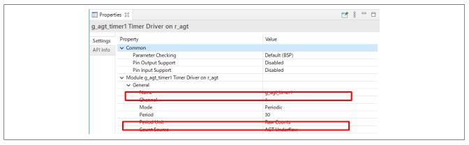
Figure 25. AGT Count Source Settings in FSP Configurator
