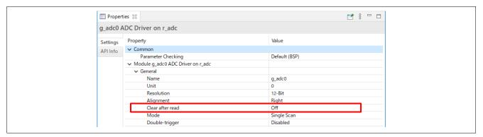
Figure 16. DC Data Register Auto Clearing Function Settings in FSP Configurator
