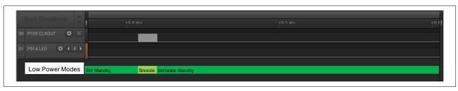
Figure 41. Example of Pin Output in Snooze Mode
