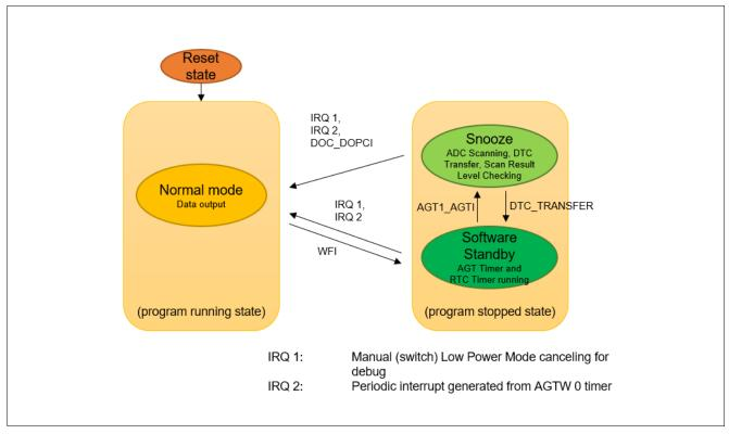
Figure 3. RA2E2 MCU Status and Mode Transition Events
