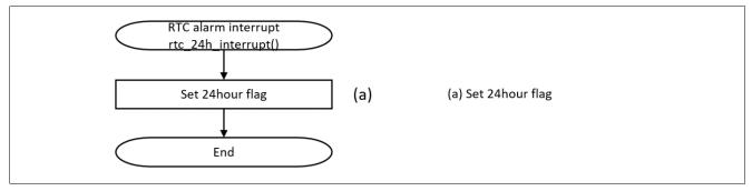
Figure 47. RTC Alarm Interrupt Processing
