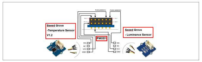
Figure 12. FPB-RA2E2 kit PMOD1 Connection with Analog Sensors
