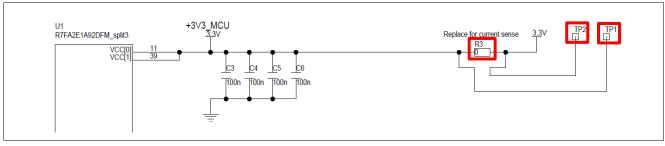
Figure 60. MCU Current Measuring Points (Circuit Diagram)
