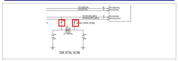
Figure 40. Solder Jumper for External Oscillator Connection (Circuit Diagram)
