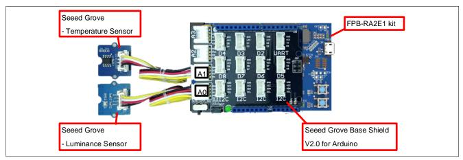
Figure 34. FPB-RA2E1 Sensor Connection
