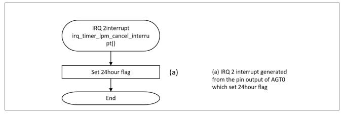
Figure 48. RA2E2 IRQ 2 Interrupt Processing
