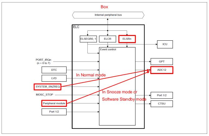
Figure 22. ELC Event Connection for ADC Start Conversion
