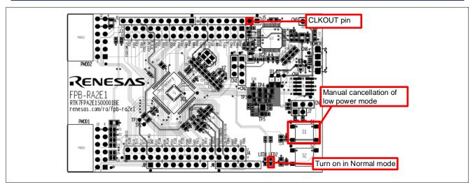
Figure 38. Debugging I/O Pins
