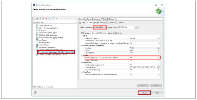
Figure 53. Debug Configuration
