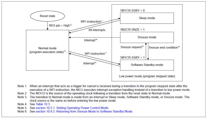
Figure 8. Schematic Diagram of Low Power Mode Transitions
