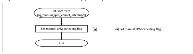
Figure 49. IRQ Interrupt Processing
