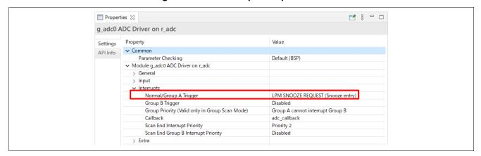
Figure 15. A/D convert Start Trigger Event Settings in FSP Configurator
