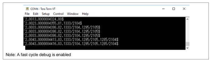
Figure 58. FPB-RA2E1 Example of Data Output Triggered by Pressing the User Switch
