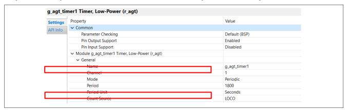
Figure 28. AGT1 Count Source Settings in FSP Configurator
