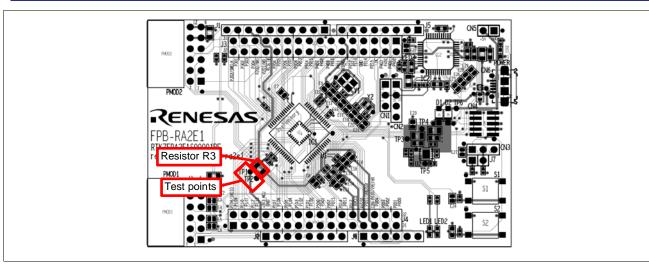
Figure 61. MCU Current Measuring Points
