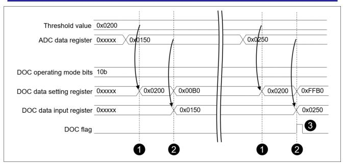
Figure 21. Level Judgement using DOC Subtraction Mode
