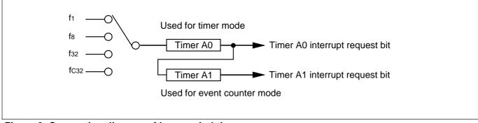
Figure 2. Connection diagram of long-period timers
