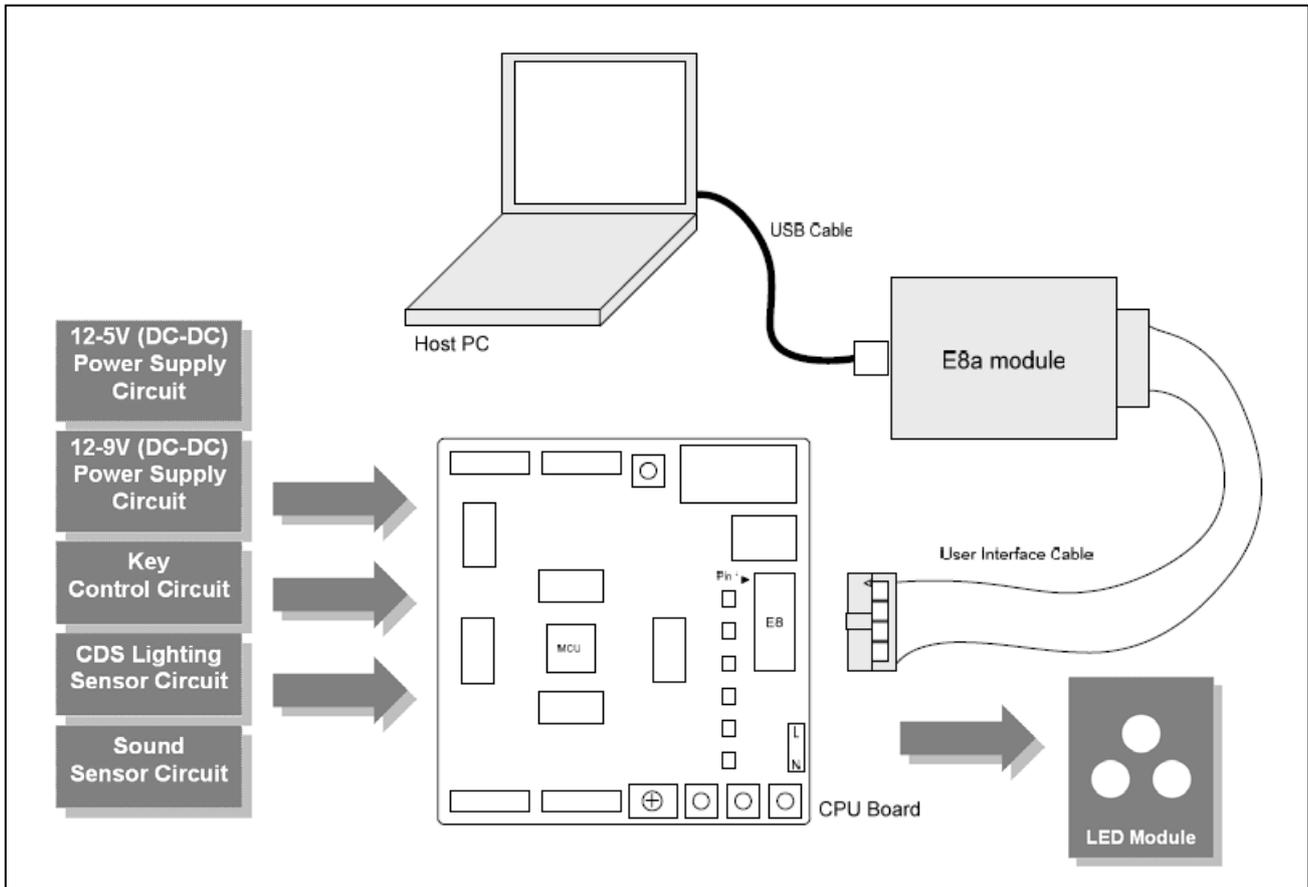
**Figure 2 Implement LED table lighting application on RSK R8C/2D**
