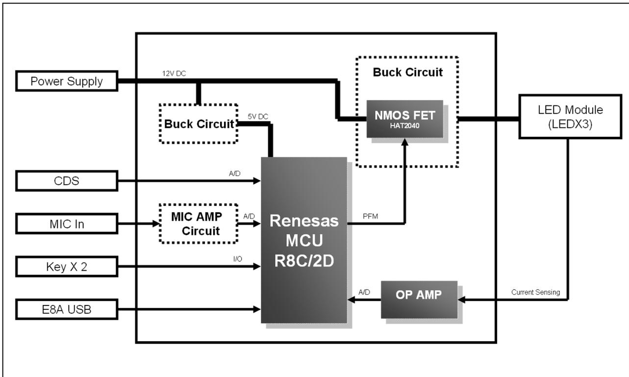
Figure 1 the configuration of the system
