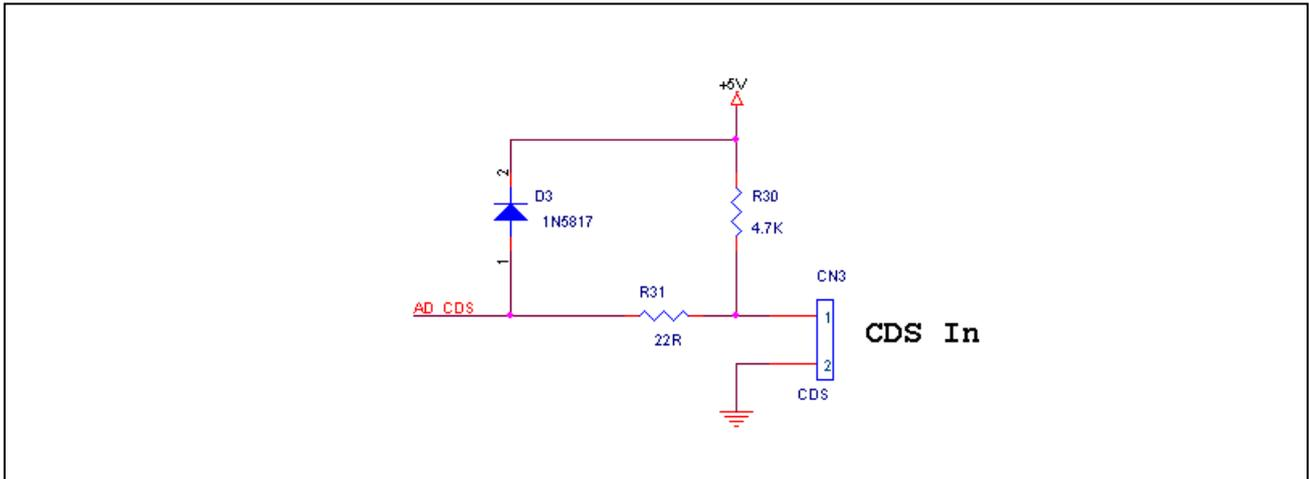
**Figure 10 CDS Sensing Circuit**
