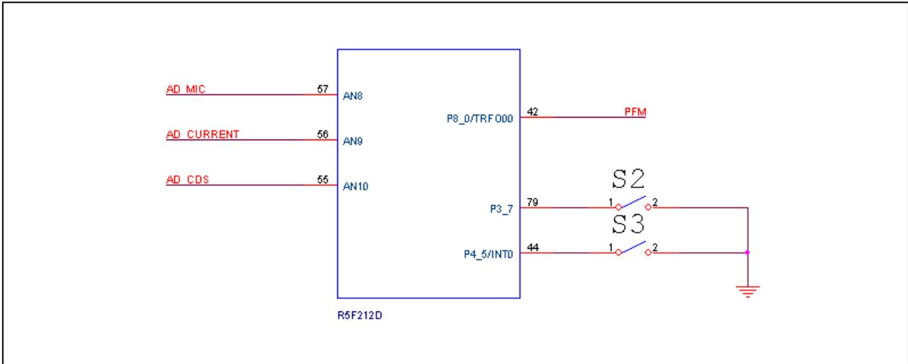
**Figure 6 R8C/2D Control Schematics**
