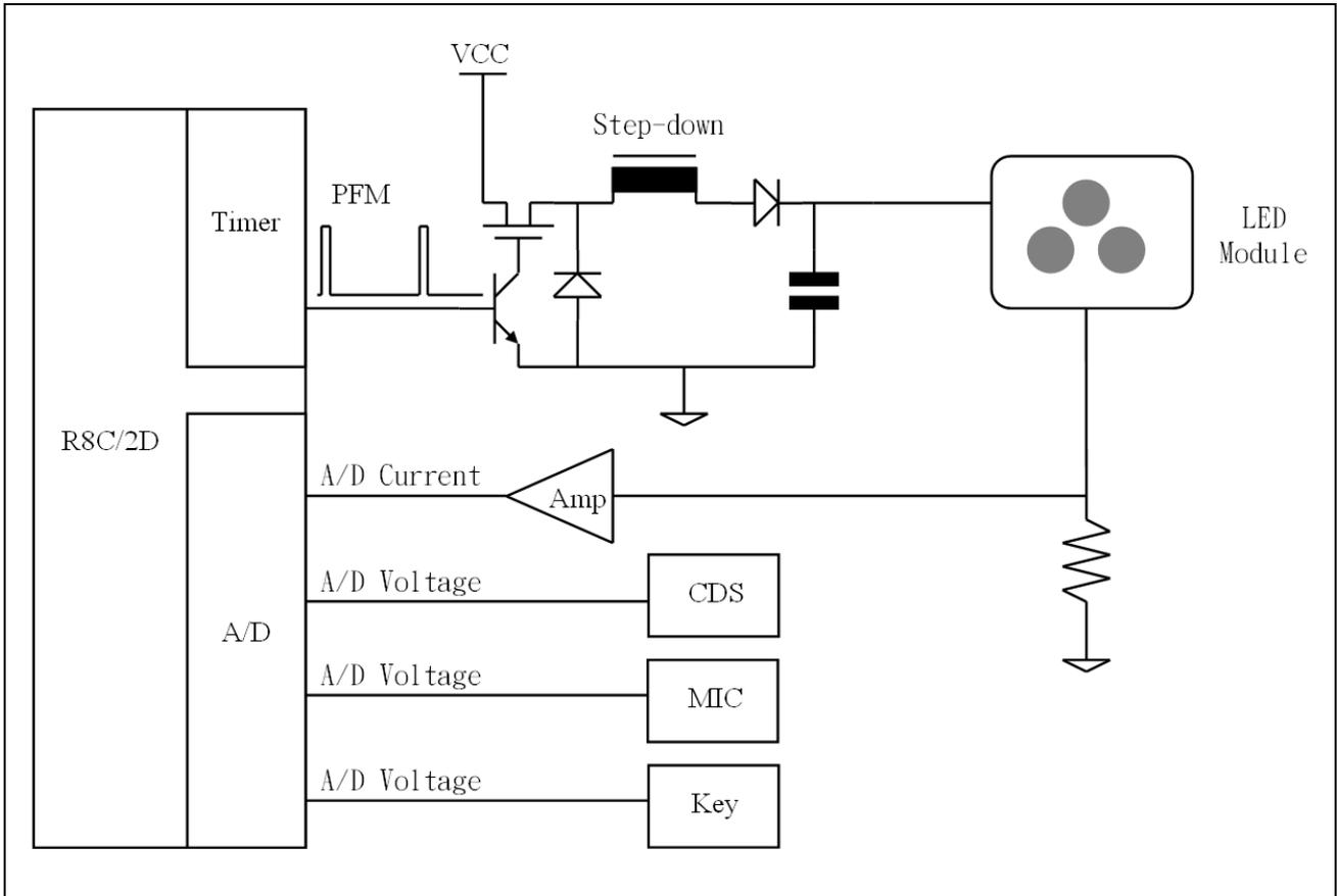
Figure 3 R8C/2D Timer RF out PFM Circuit
