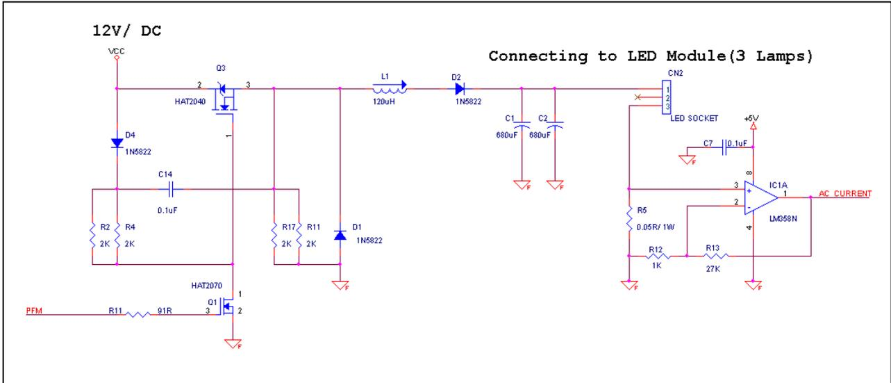
Figure 8 PFM Control Circuit
