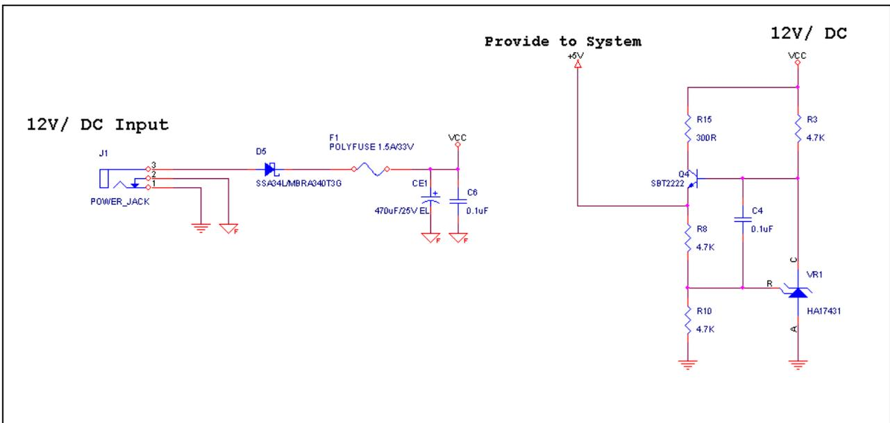
**Figure 7 System Power Supply**
