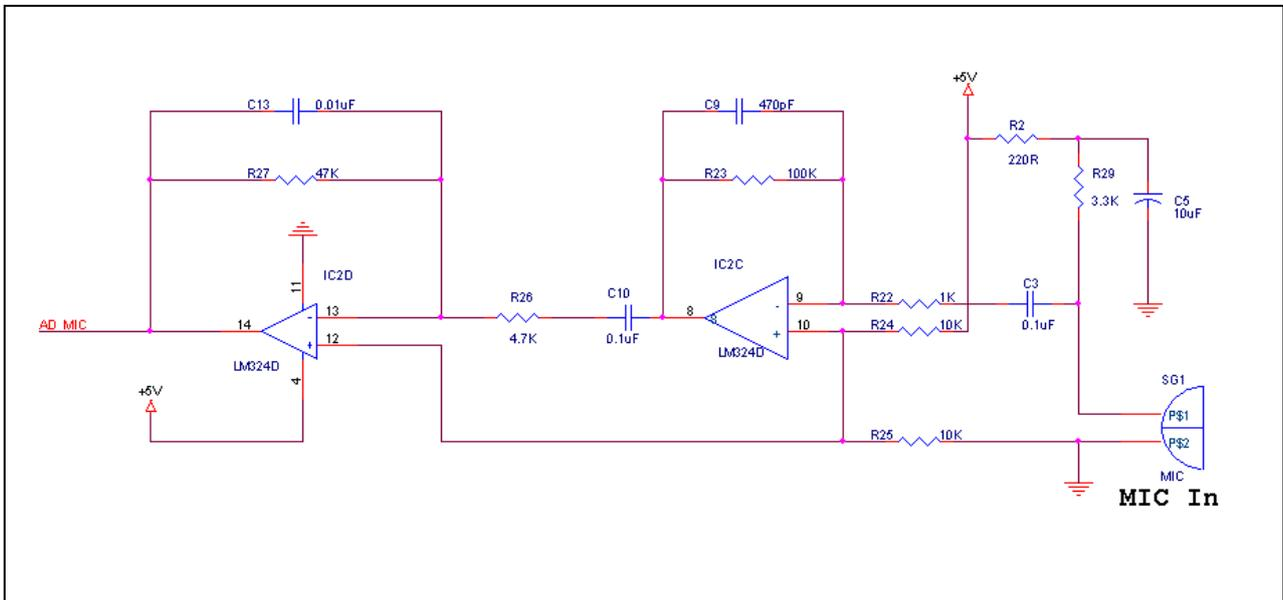
Figure 9 MIC in Sensing Circuit
