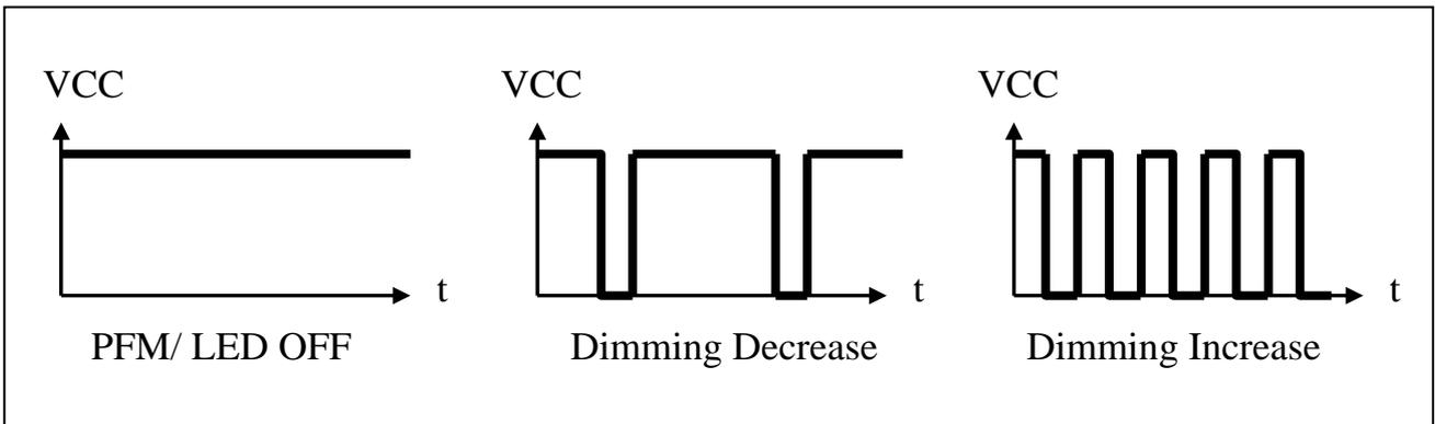
Figure 4 PFM Dimming Signals
