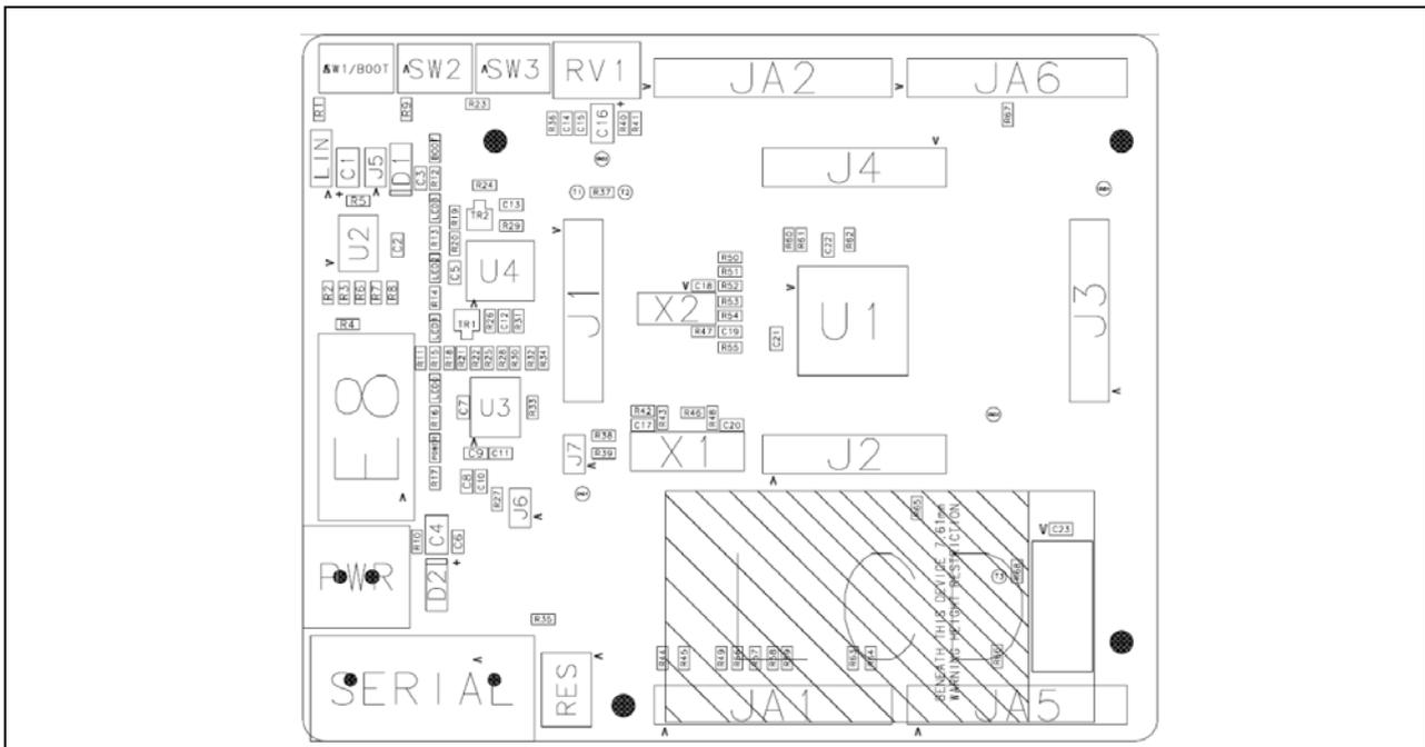
**Figure 5 Connectors placement of Renesas Starter Kit CPU Board for R8C/2D**
