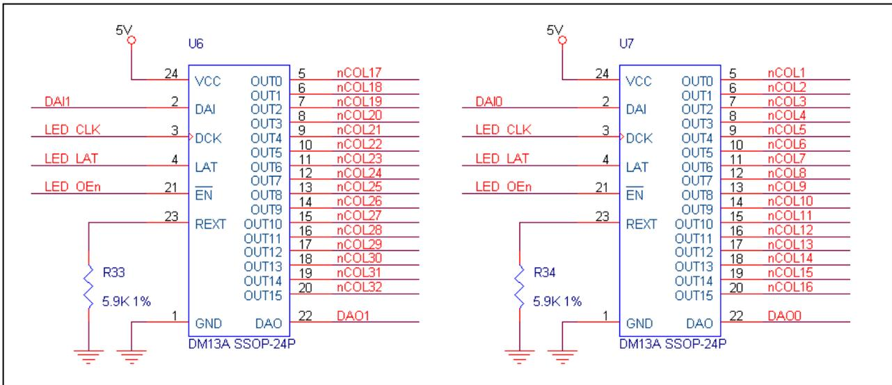
Figure 9 Serial to Parallel Shifter of Column Data (2)
