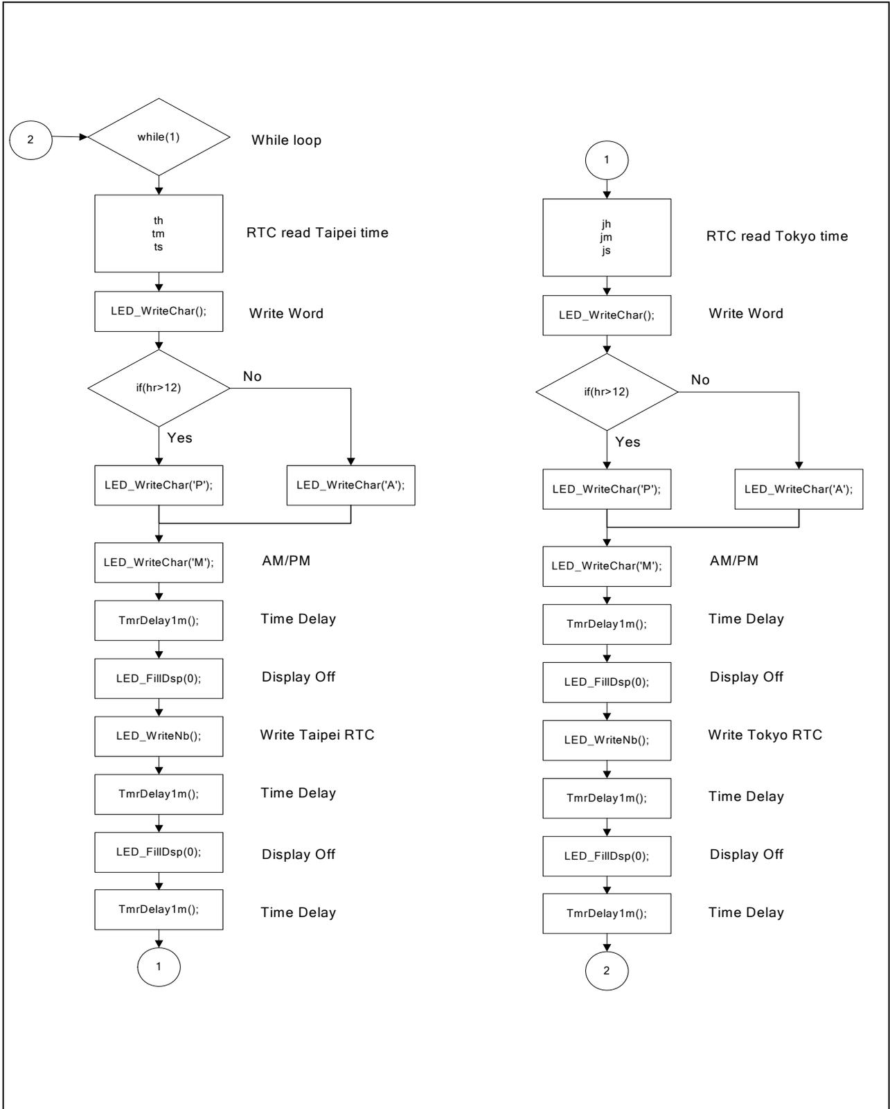
Figure 16 Program flow chart of while(1) loop routine
