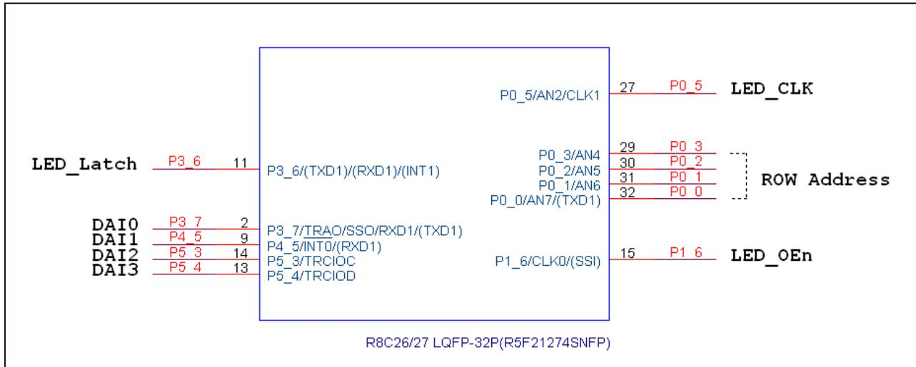
Figure 7 R8C/27 Control Schematics
