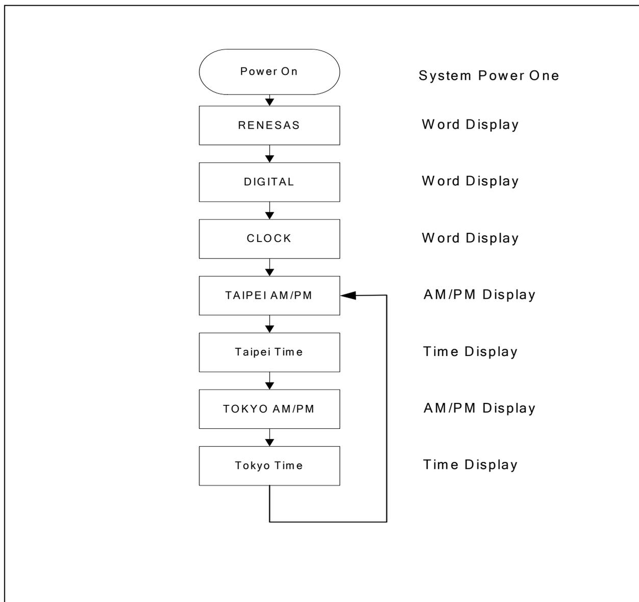
Figure 14 Demo flow chart of LED Digital Clock
