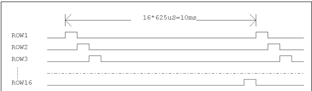
Figure 5 Row Scan Line Timing
