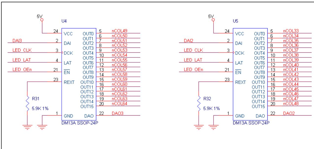
Figure 8 Serial to Parallel Shifter of Column Data (1)
