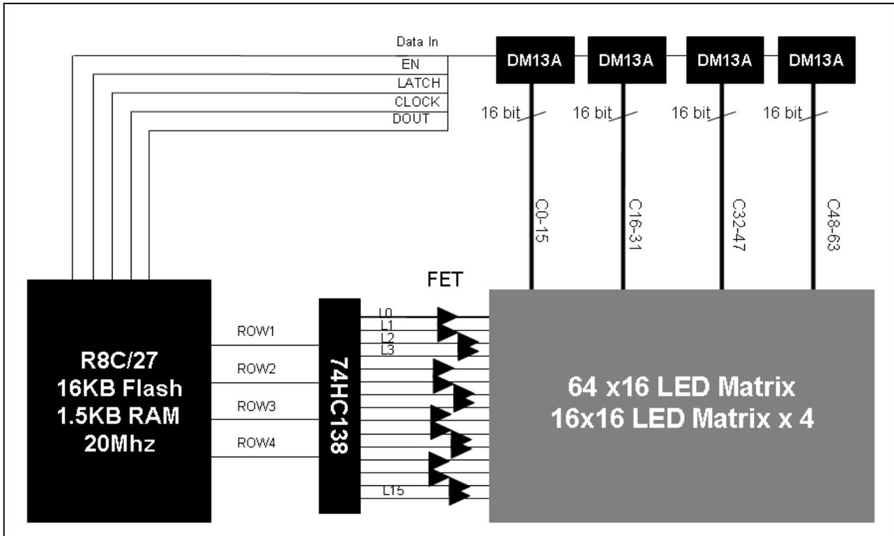
Figure 1 The configuration of the system
