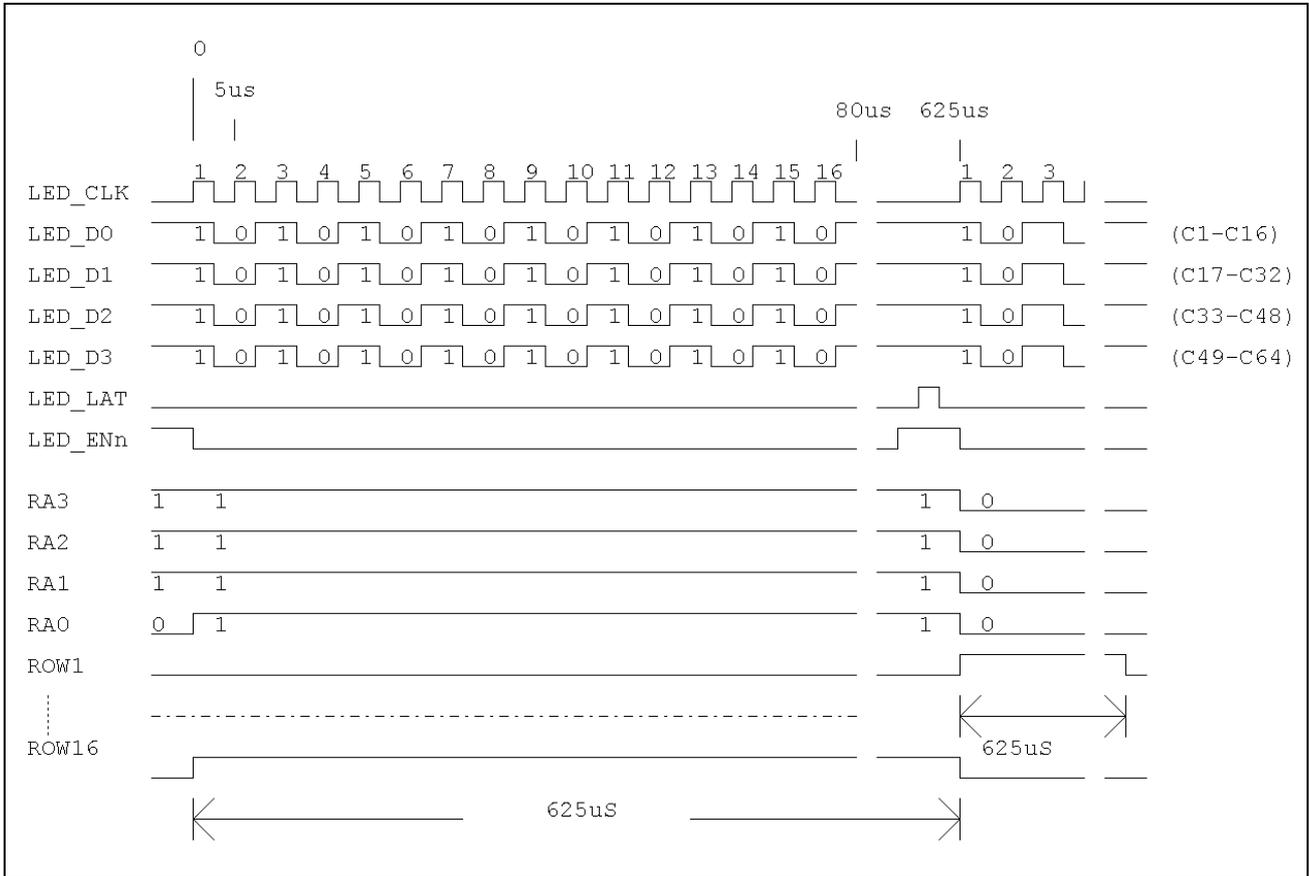
Figure 4 Column Data Shifter Timing
