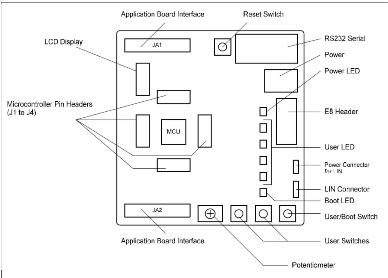
Figure 6 Connectors placement of Renesas Starter Kit CPU Board for R8C/27
