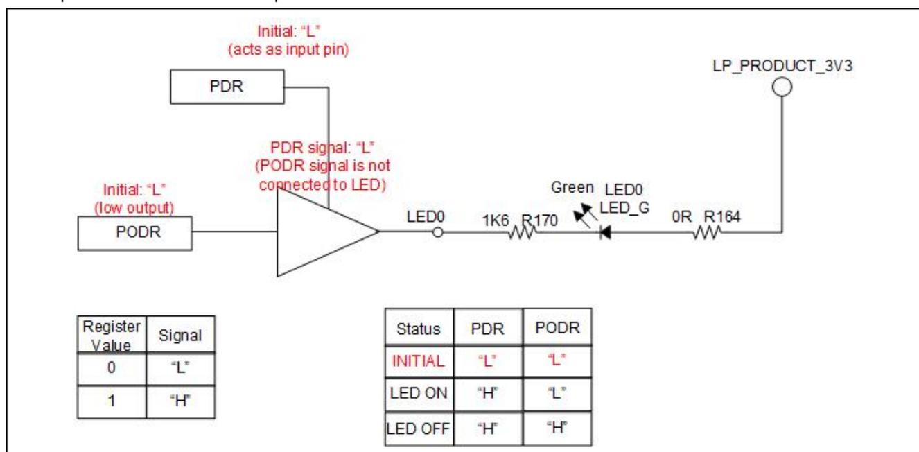
**Figure 1.1 LED Pin Schematic Diagram**
