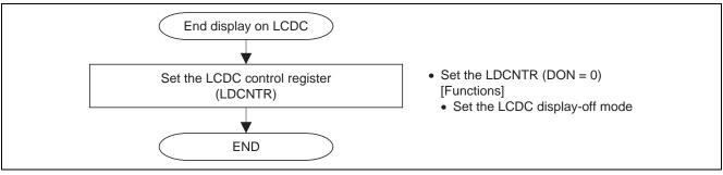
Figure 14 Setting Examples of the Stop of LCDC Display
