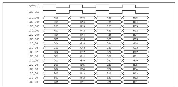
Figure 4 Clock and LCD Data Signal Example (TFT Color 16-Bit Data Bus Module)
