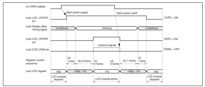
Figure 5 Power-Supply Control Sequence and States of the LCD Module
