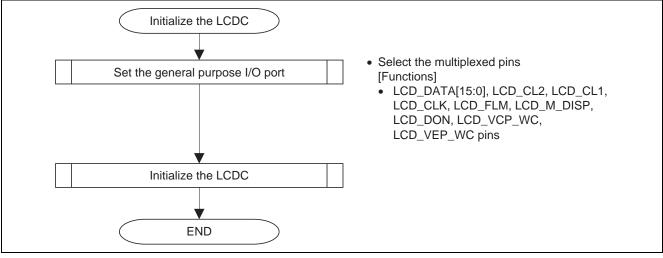
Figure 10 Flow for Initialization of the LCDC
