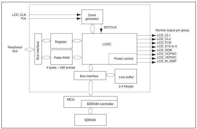
Figure 1 LCDC Block Diagram
