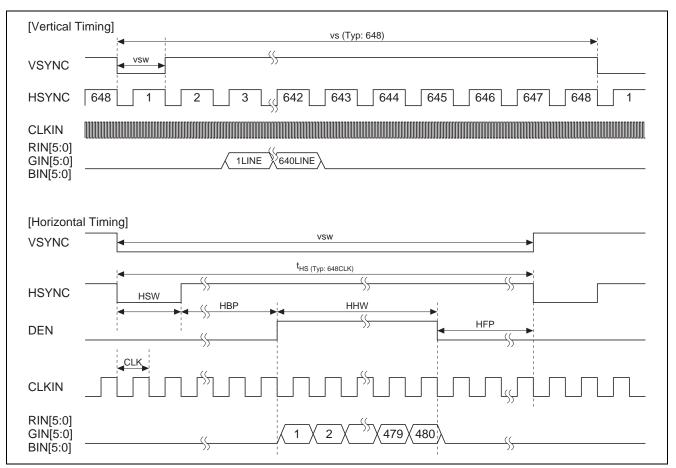
Figure 6 TFT-LCD Panel Interface Timing Example (Excerpt from Datasheet)
