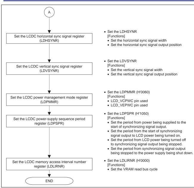
Figure 12 Setting Examples of the LCDC (2)
