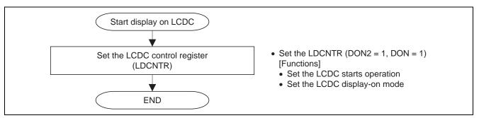
Figure 13 Setting Examples of the Start of LCDC Display
