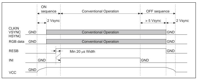
Figure 7 TFT-LCD Panel Power-Supply Sequence (Excerpt from Datasheet)
