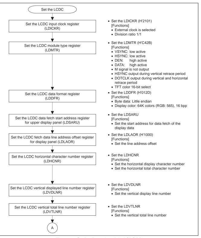
Figure 11 Setting Examples of the LCDC (1)
