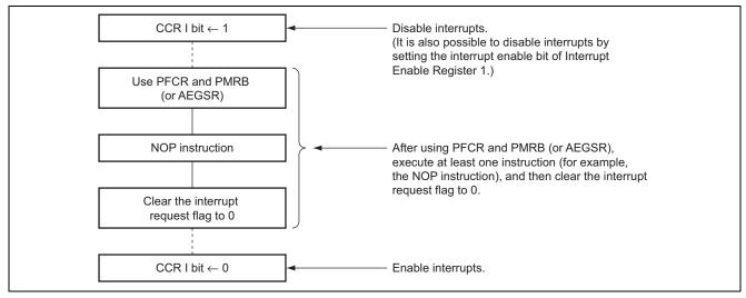
Figure 2 Procedure for Manipulating PFCR and PMRB (or AEGSR) and Clearing the Interrupt Request Flag
