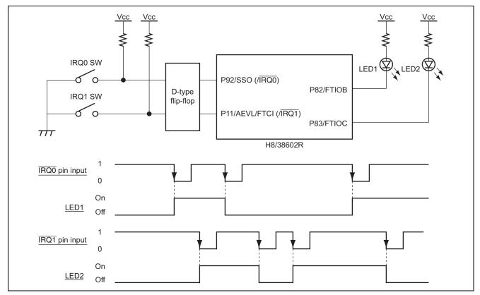
Figure 1 Setting of the IRQ Pins
