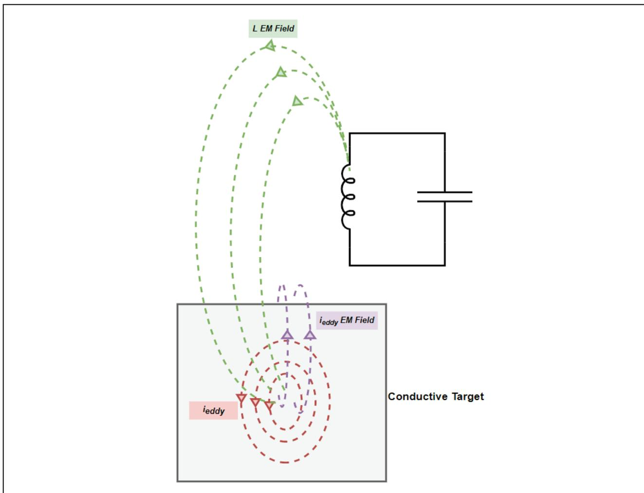
**Figure 5. Electric Field Lines**
