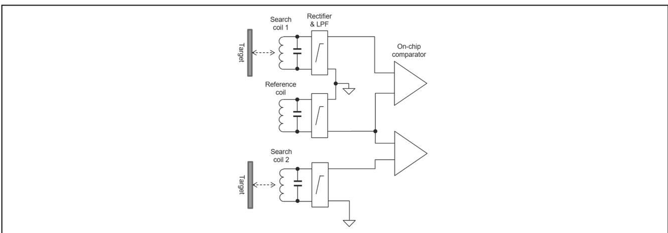
**Figure 13. Simultaneous Sensing**
