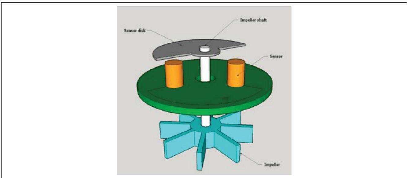
Figure 16. Rotational liquid flow sense with multiple sensors
