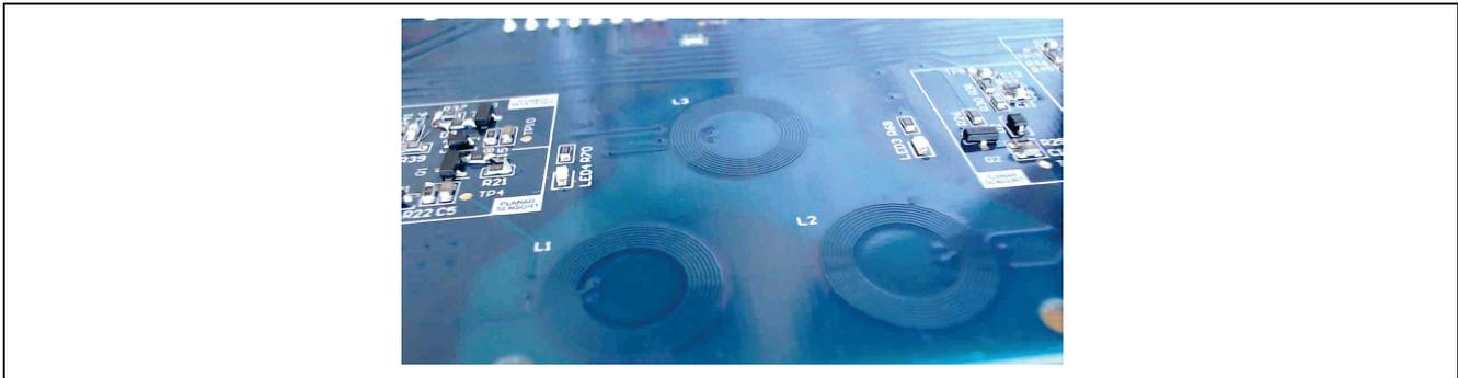
**Figure 12. Air-cored Planar Inductor**
