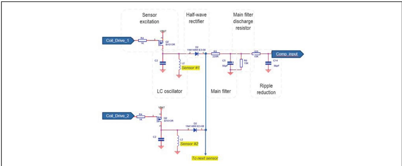
**Figure 14. Sequential Sensing (search coil - OR diode)**
