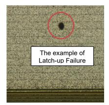
Figure 4-2 Representative failure mode
