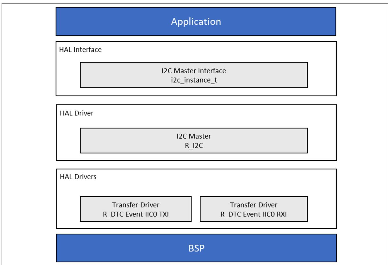
Figure 1 I<sup>2</sup>C Master HAL Module Block Diagram
