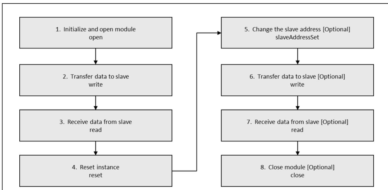
Figure 3 Flow Diagram of a Typical I<sup>2</sup>C Master HAL Module Application
