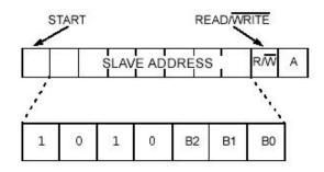
The next three bits of the control byte are the block select bits (B2, B1, B0). They are used by the master device to select which of the eight 256 word blocks of memory are to be accessed. These bits are in effect the three most significant bits of the word address.
