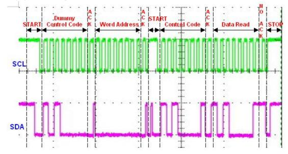
The average time for reading a byte of data using random read operation is \*22.3ms.
