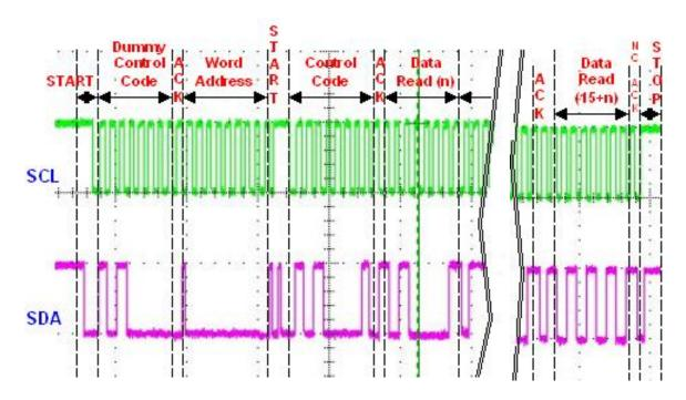
The average time for reading a page of 16kbytes using sequential read operation is \*97.8ms.
