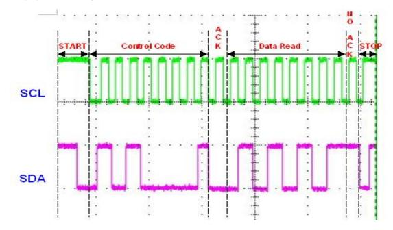
The average time for reading a byte using current read operation is \*11.2ms.
