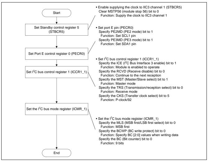
Figure 2 IIC3 Configuration Flow Chart
