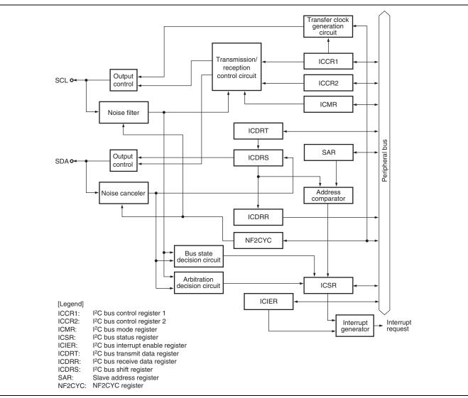
Figure 1 IIC3 Block Diagram
