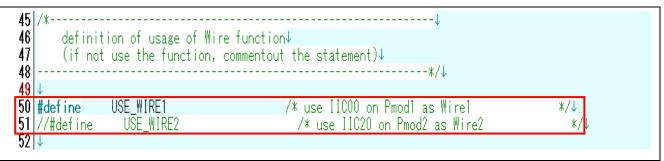
Figure 1.2 Lines where the WireAPI function to be used is defined
