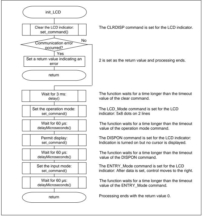
Figure 5.6 LCD Indicator Initialization Function
