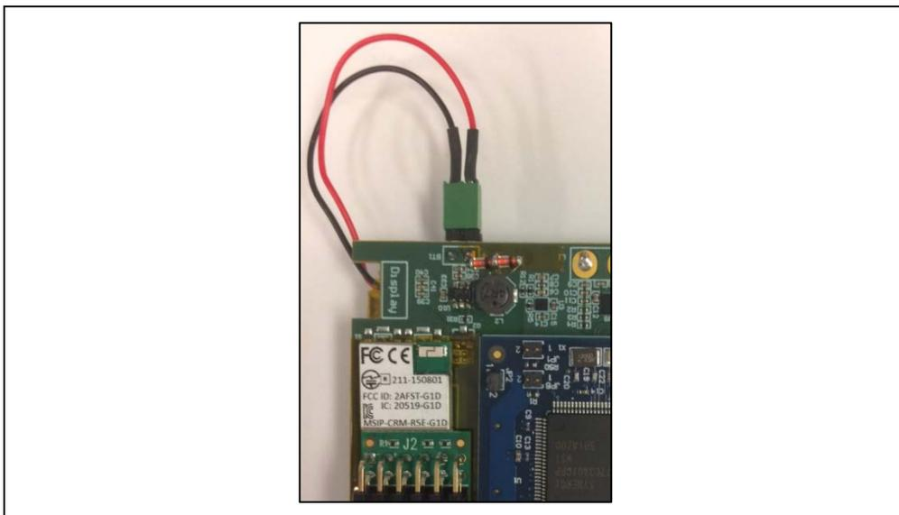
**Step 4.** If battery power is diminished, connect to Qi wireless charging pad to charge the battery. Other option to charge the battery is to power the board using USB port.
