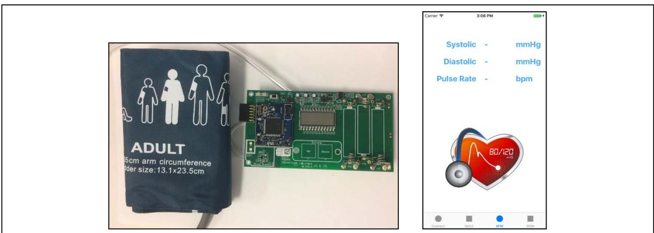
Figure 3-3 Blood Pressure Module with Mobile App snapshot
