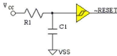
**Figure 2.1 Reset circuit I**
