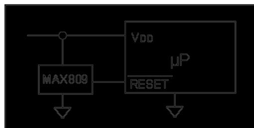
Figure 2.4 Reset Circuit IV with Maxim IC (MAX809)
