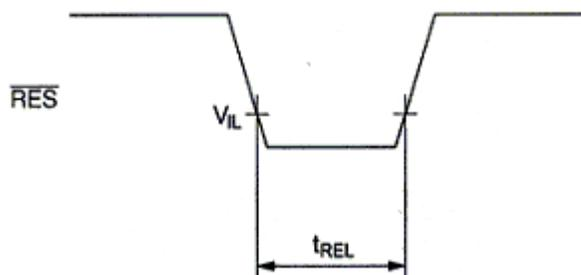
Figure 1.2 Reset Low Width
