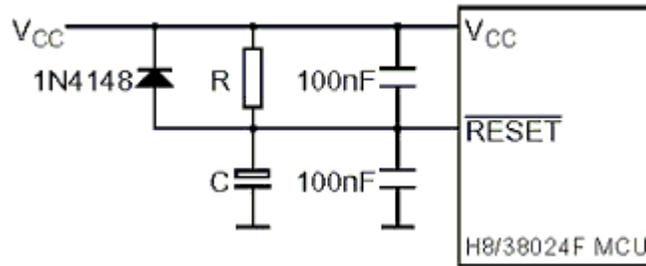
Figure 2.3 Reset Circuit III with a Discharge Diode
