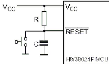
Figure 2.2 Reset Circuit II
