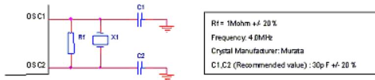
**Figure 3.2 Connection to Ceramic Oscillator**
