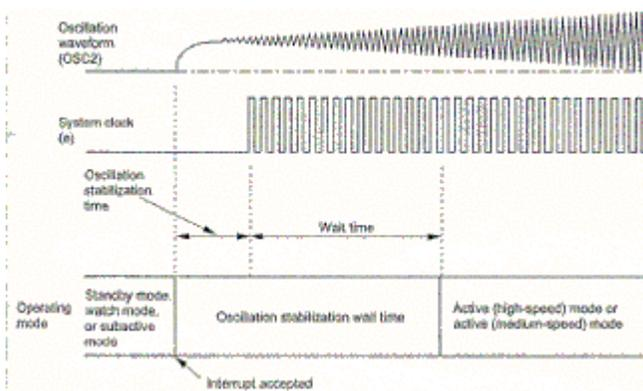
Figure 6.1 Oscillation Stabilization Time
