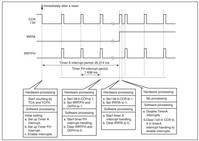
Figure 3.1 Operation Principle of Multiple-Interrupt Handling for Internal Interrupts
