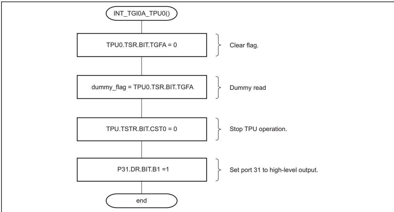
Figure 10 Flowchart (DTC End Interrupt)
