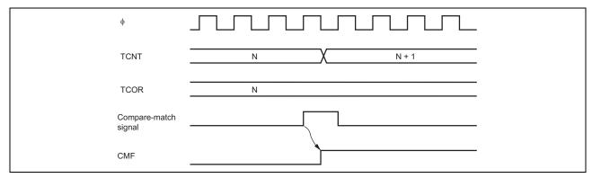
Figure 3 Timing of CMF Setting at Compare-Match
