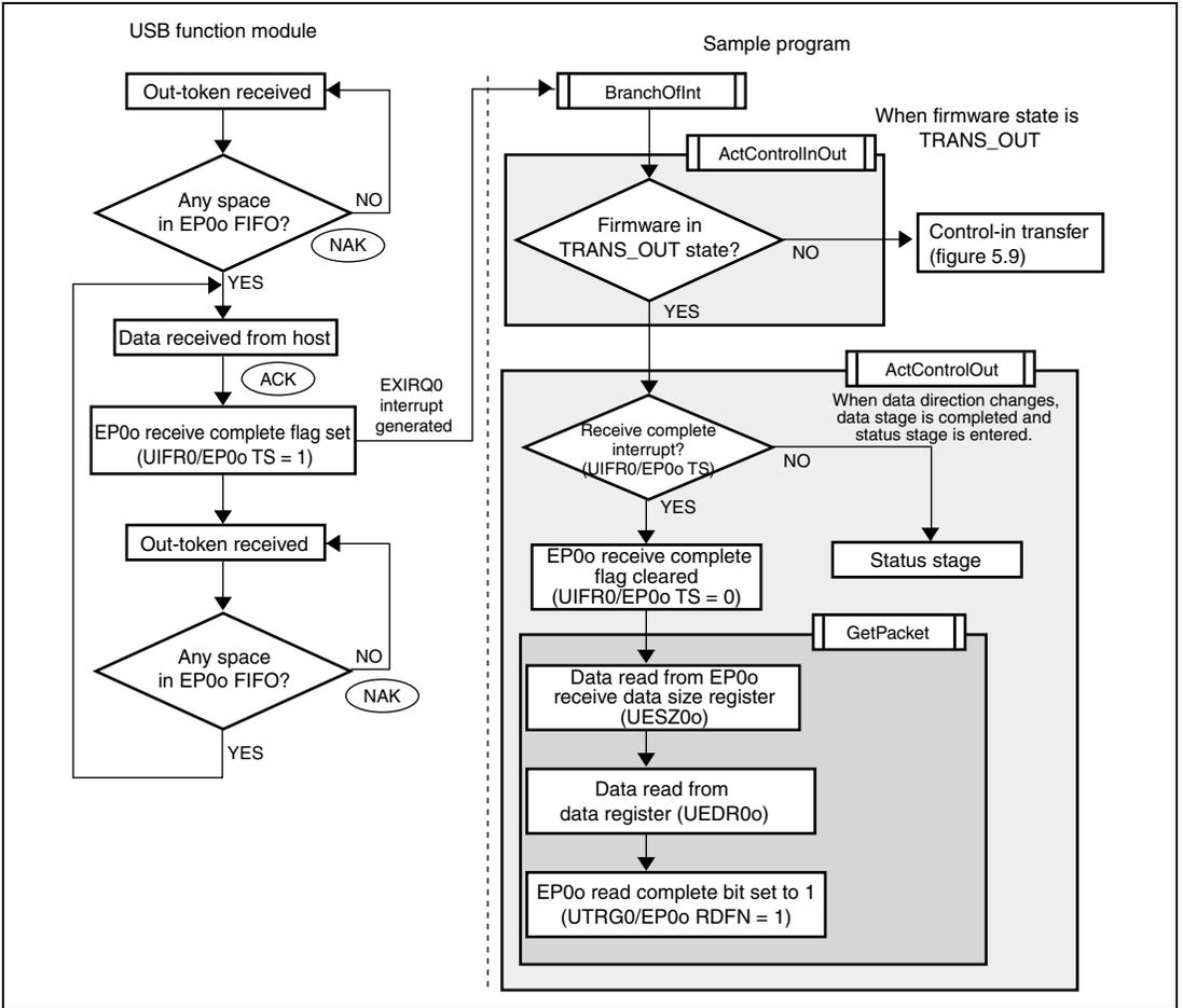
**Figure 5.10 Data Stage (Control-Out Transfer)**
