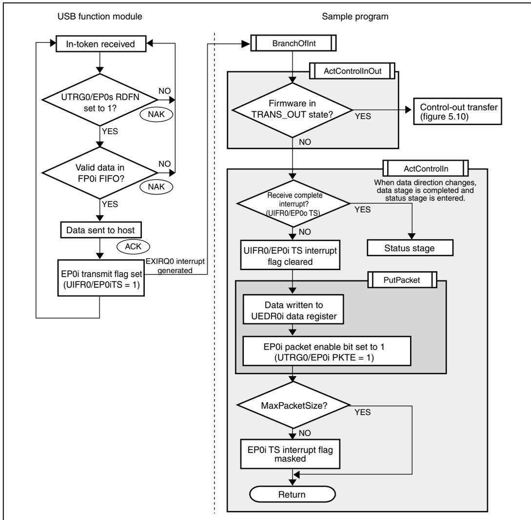
Figure 5.9 Data Stage (Control-In Transfer)
