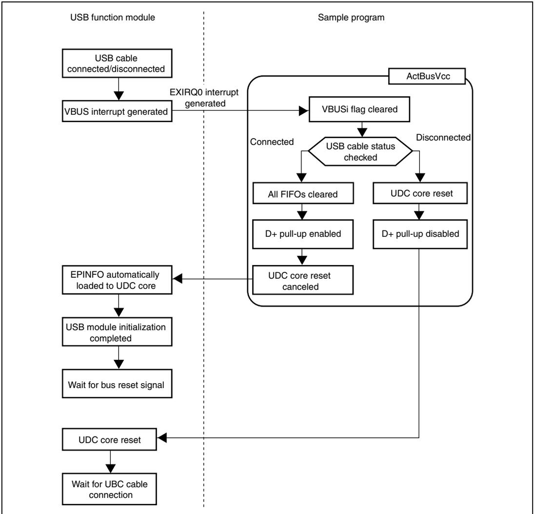
Figure 5.4 Interrupt on Cable Connection
