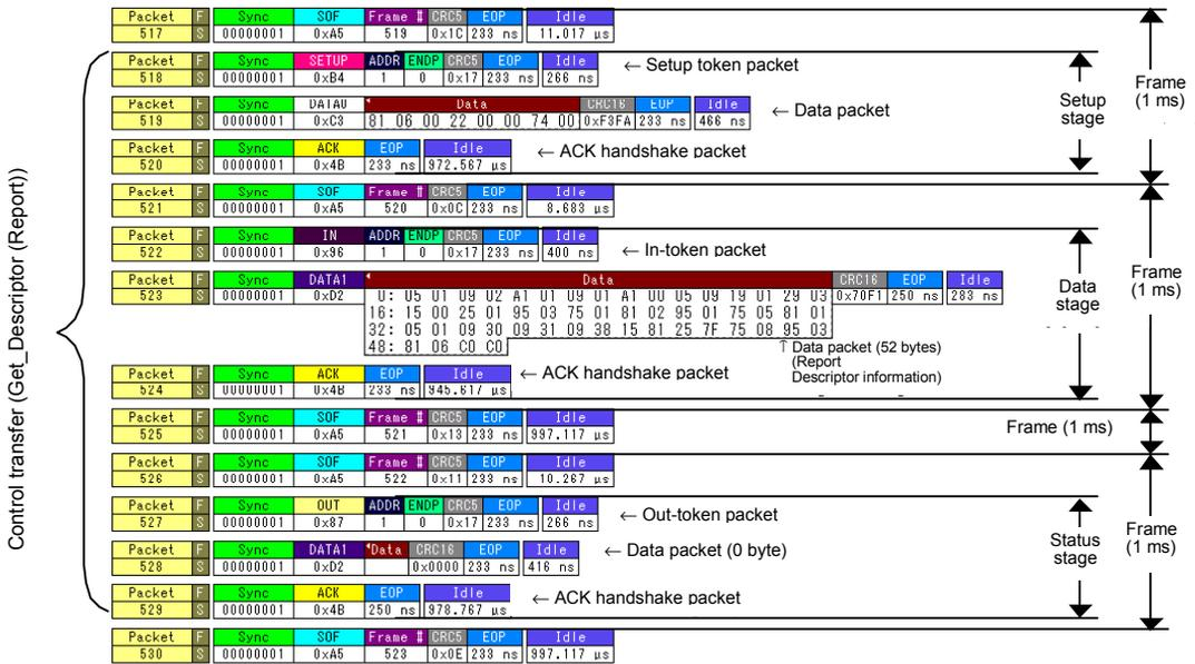
Figure 6.1 Control Transfer when Device is Connected
