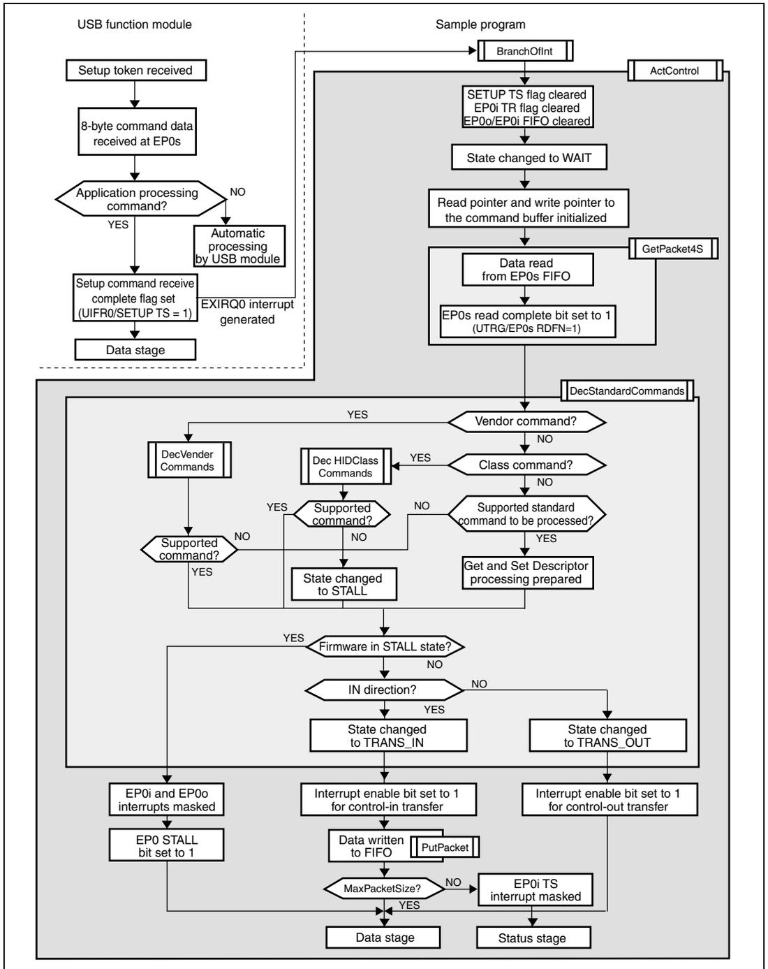
Figure 5.8 Setup Stage
