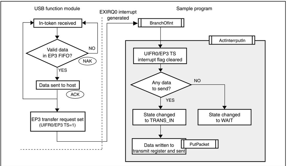
**Figure 5.14 Interrupt-In Transfer**
