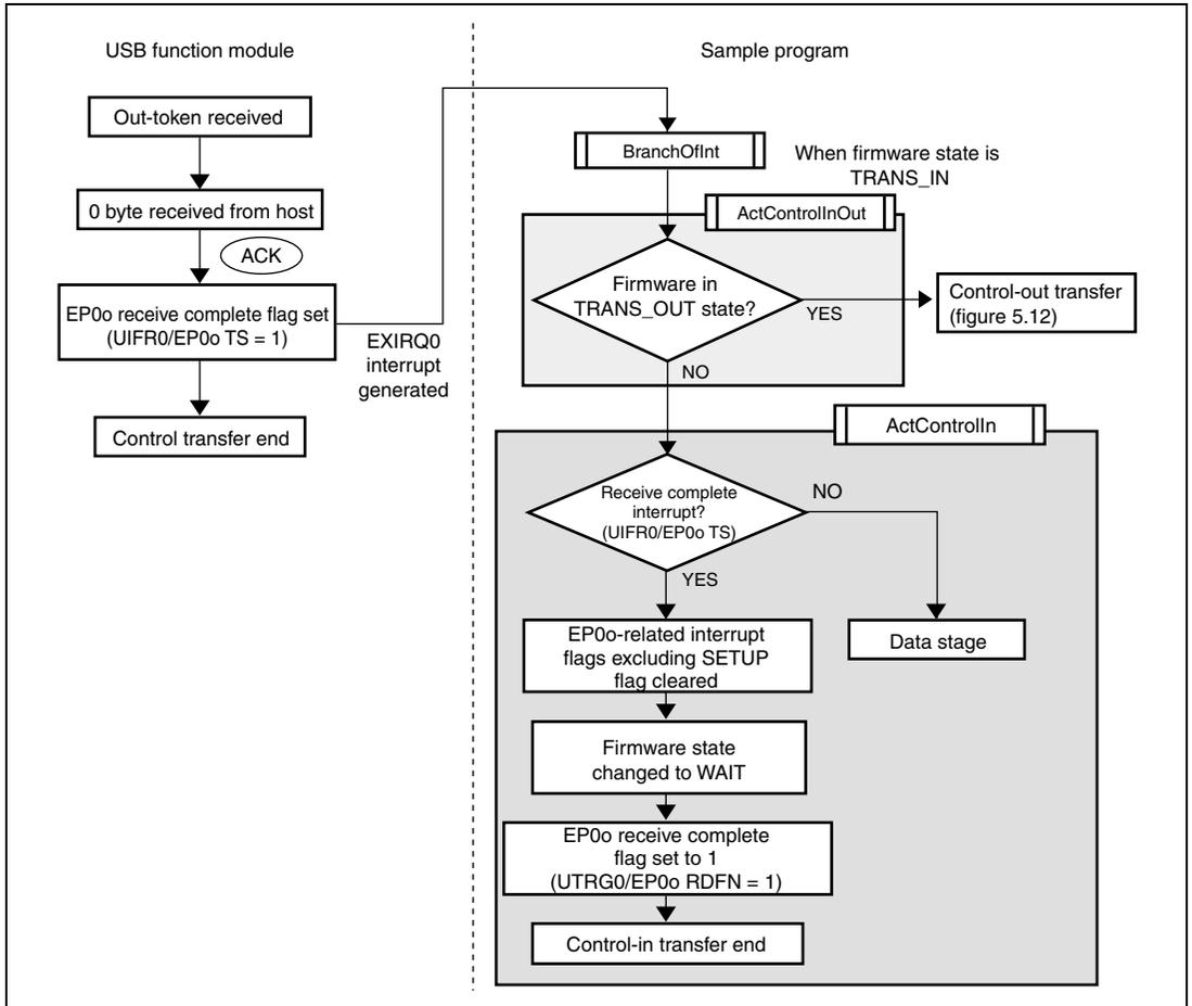
**Figure 5.11 Status Stage (Control-In Transfer)**
