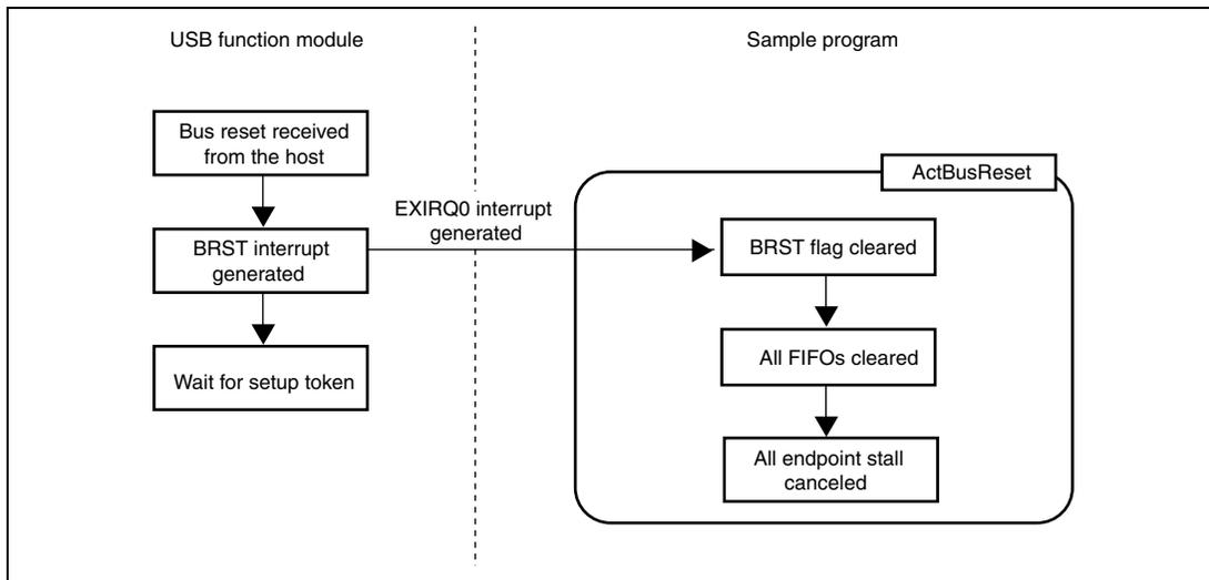
**Figure 5.5 Bus Reset Interrupt**
