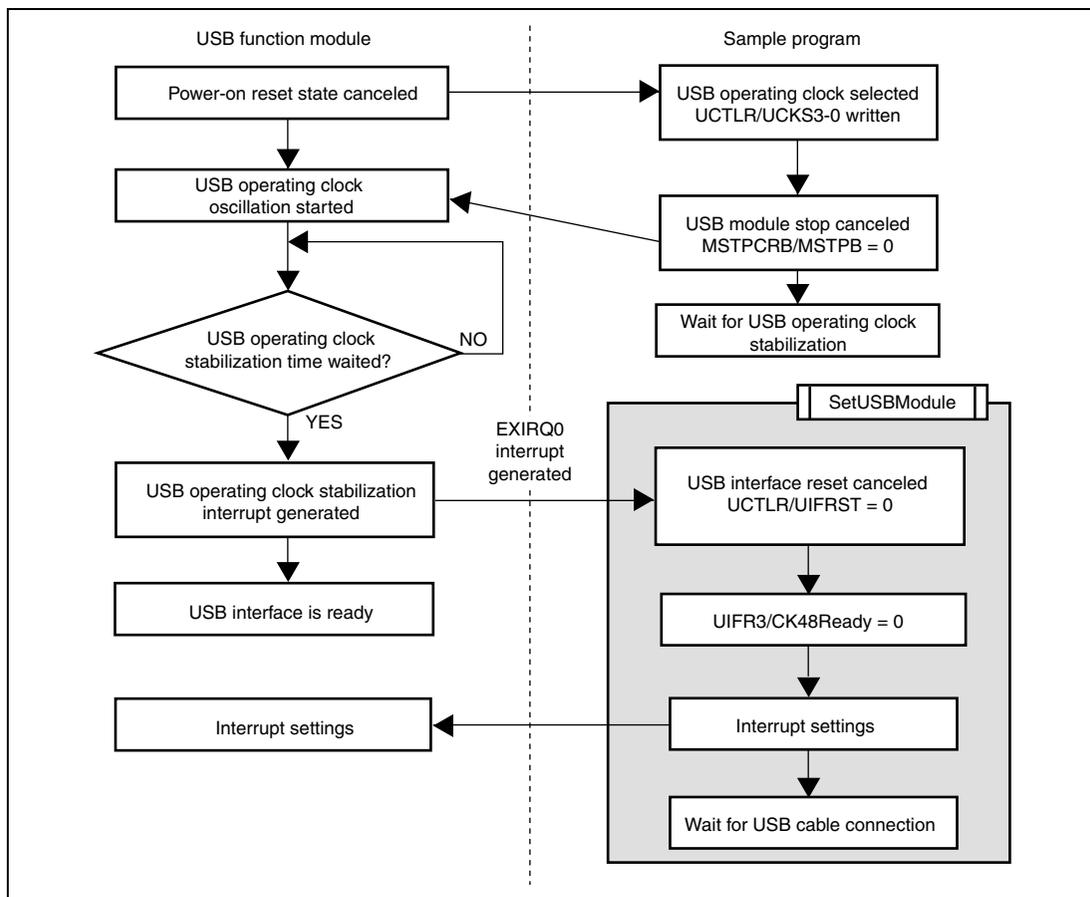
Figure 5.3 USB Operating Clock Stabilization Interrupt
