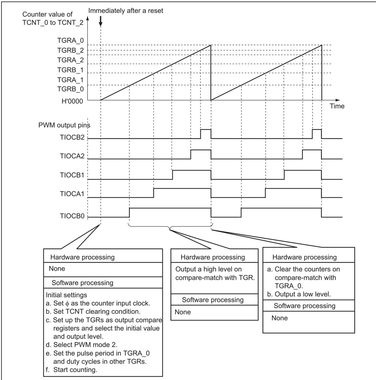
Figure 3 PWM Pulse Output Operation
