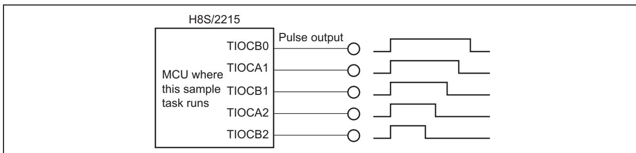
**Figure 1.1 Example of PWM Pulse Output**
