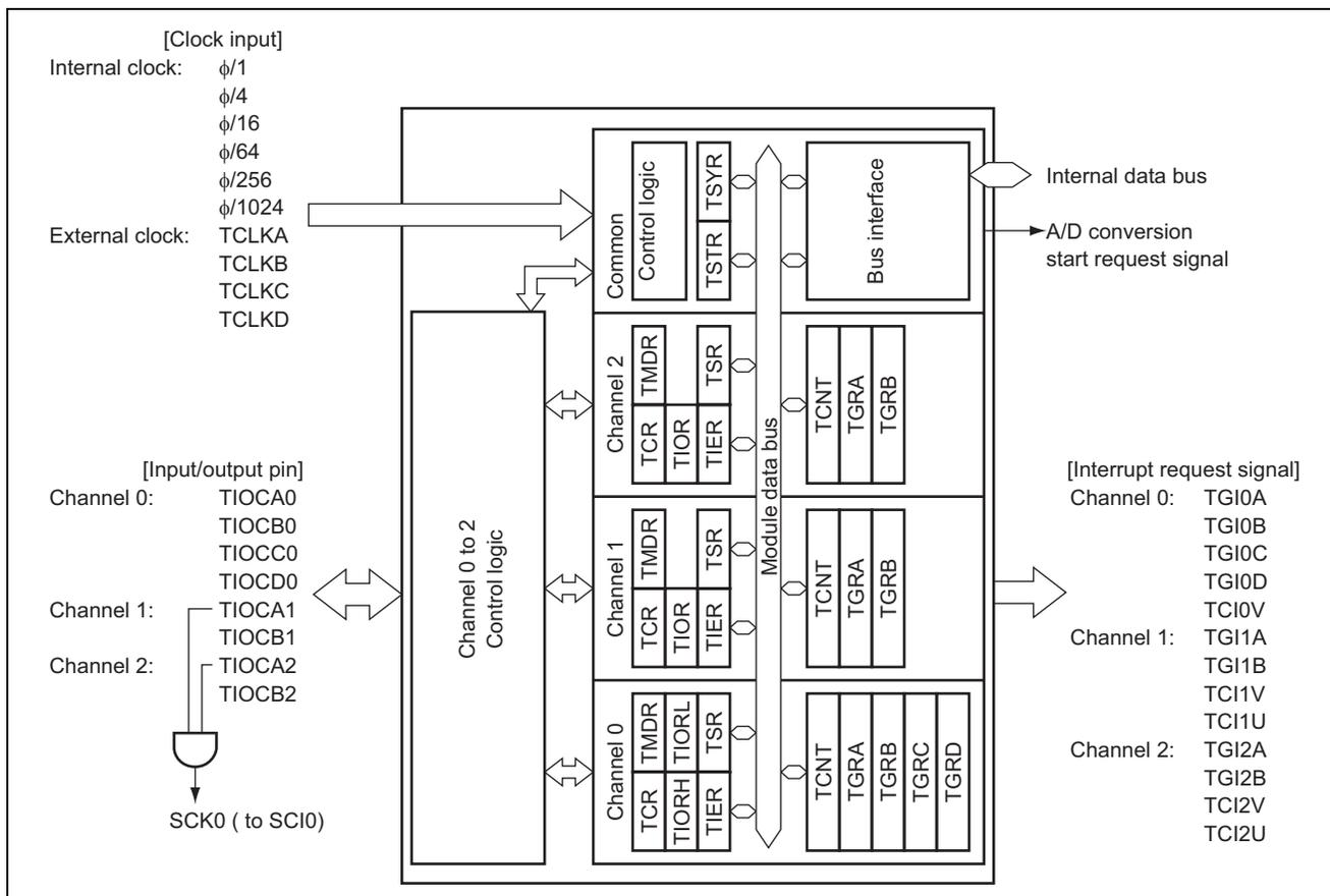
**Figure 2.1 Block Diagram of TPU**
